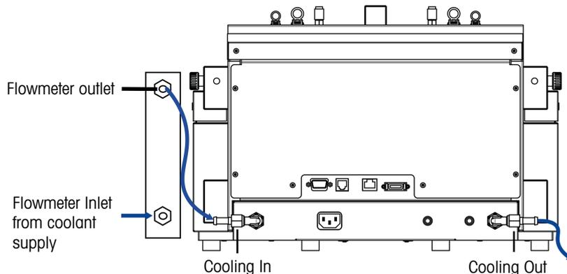
The instrument is delivered with two PVC industrial tubes. If you use the flowmeter, you need a third piece which can be cut away from one of the delivered tubes.
