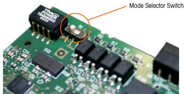
**Figure A-84: Discrete I/O Mode Selector Switch, Active Position**
