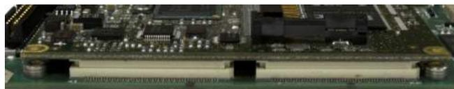
**Figure 4-58: ETX Board Resting on Connectors**
