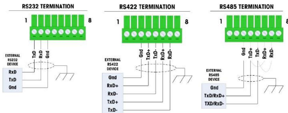
**Figure A-93: Connector Terminations for Serial Option Board**
