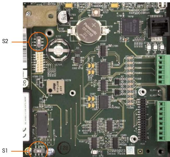
**Figure A-37: Main PCB Switch Locations**
