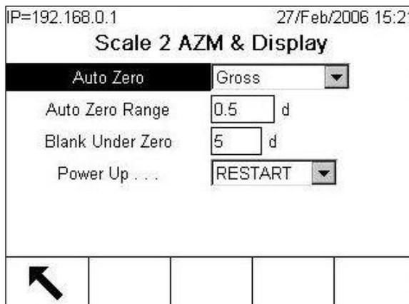
**Figure 3-44: AZM and Display Screen**
