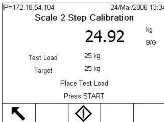
**Figure 3-31: Step Calibration, First Step Prompt**
