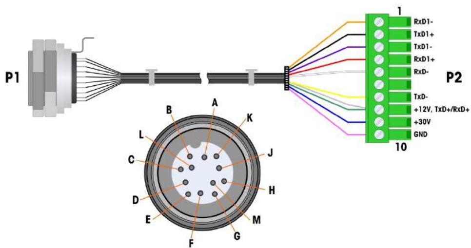
Figure A-90: IDNet Cable for IDNet Option Board
