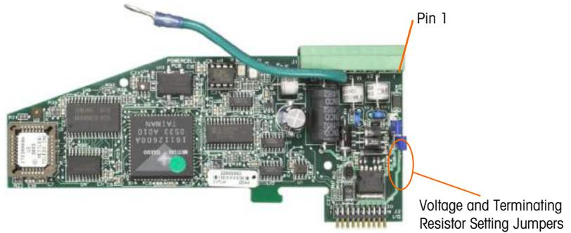
**Figure A-46: POWERCELL MTX Option Board**
