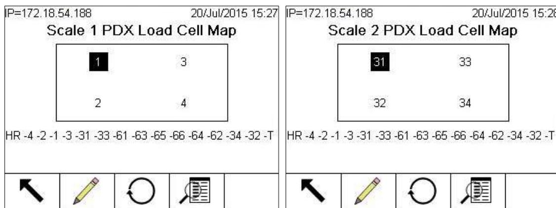
**Figure 3-177: Load Cell Maps for Scales 1 and 2, All Cells Displayed**
