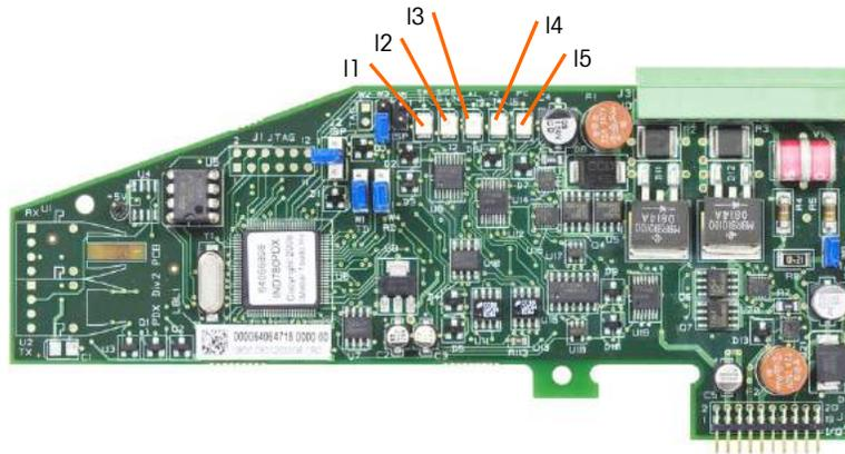
**Figure 4-11: Board LEDs**
