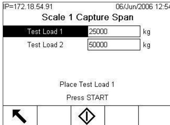
**Figure 3-29: Capture Span Screen**
