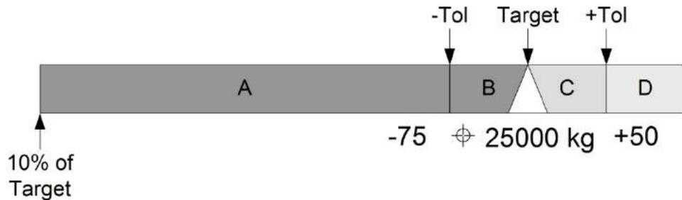
Figure 2-29: Medium Size SmartTrac Bar Graph With Display Ranges
