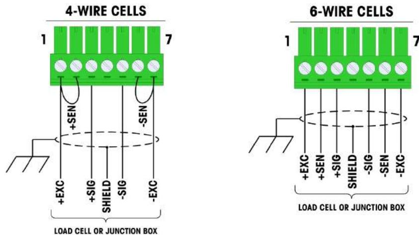
**Figure A-43: Load Cell Connections**
