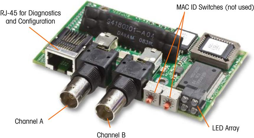
**Figure A-99: ControlNet PLC Module Connections and Components**
