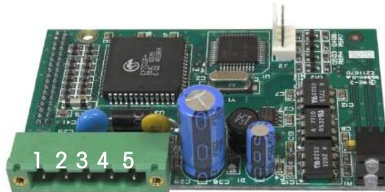
**Figure A-103: DeviceNet Option Board Connector Pin Numbering**
