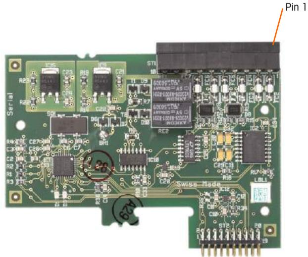
Figure A-91: Serial Option Board
