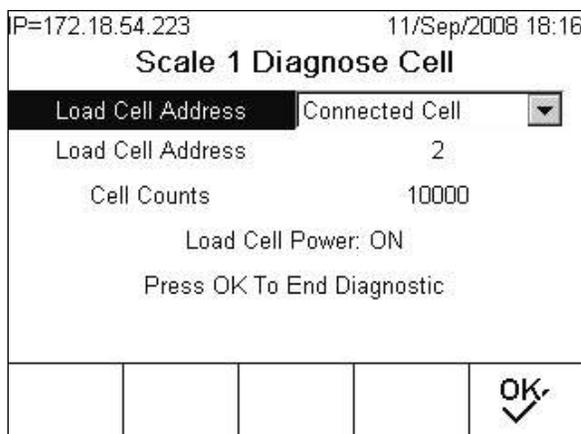
**Figure 3-206: Diagnose Cell End Diagnostic Screen**
