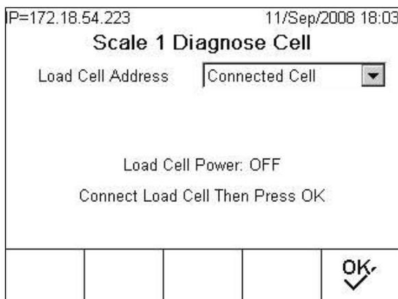
**Figure 3-205: Diagnose Cell Connect Cell Screen**
