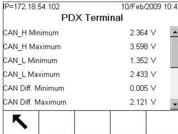
**Figure 3-198: PDX Terminal Screen**
