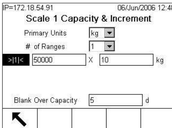
**Figure 3-24: Capacity and Increment Setup Screen**
