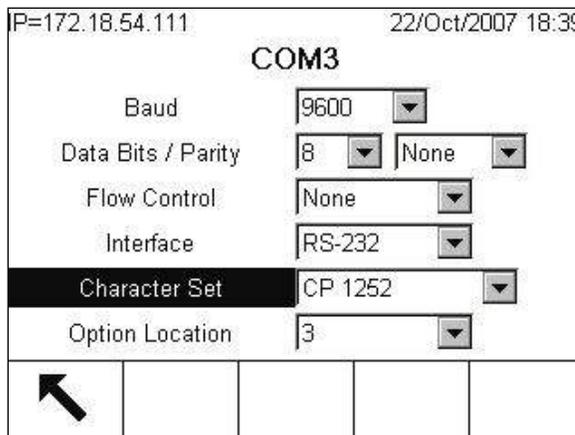
**Figure 3-121: COM3 Setup Screen**
