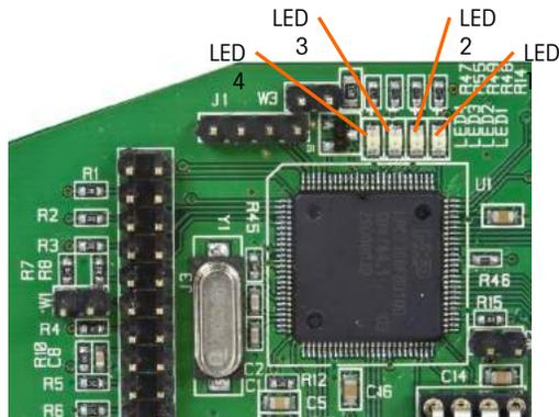
**Figure 4-12: Analog Output Board LEDs**
