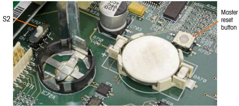
**Figure A-38: Main PCB Master Reset Button Location**
