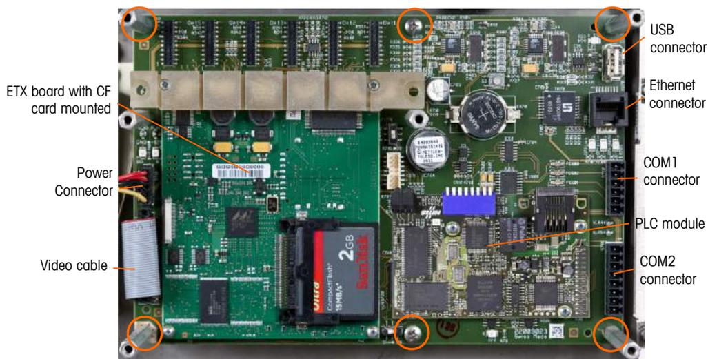
**Figure 4-52: Main PCB Connections and Mounting Screws**
