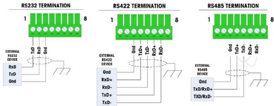
Figure A-36: COM2 Wiring for External Equipment
