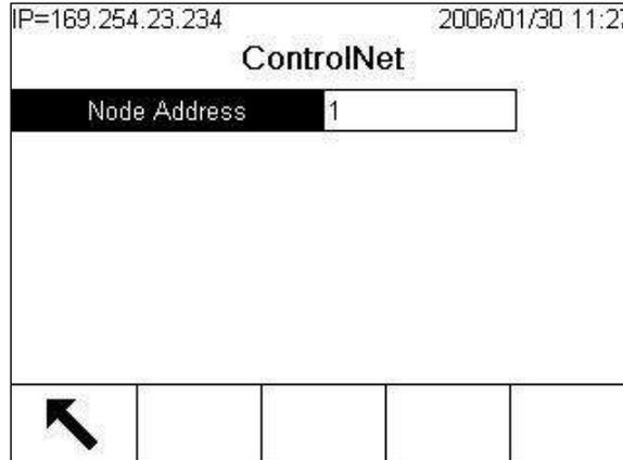
**Figure 3-139: ControlNet PLC Interface Setup Screen**
