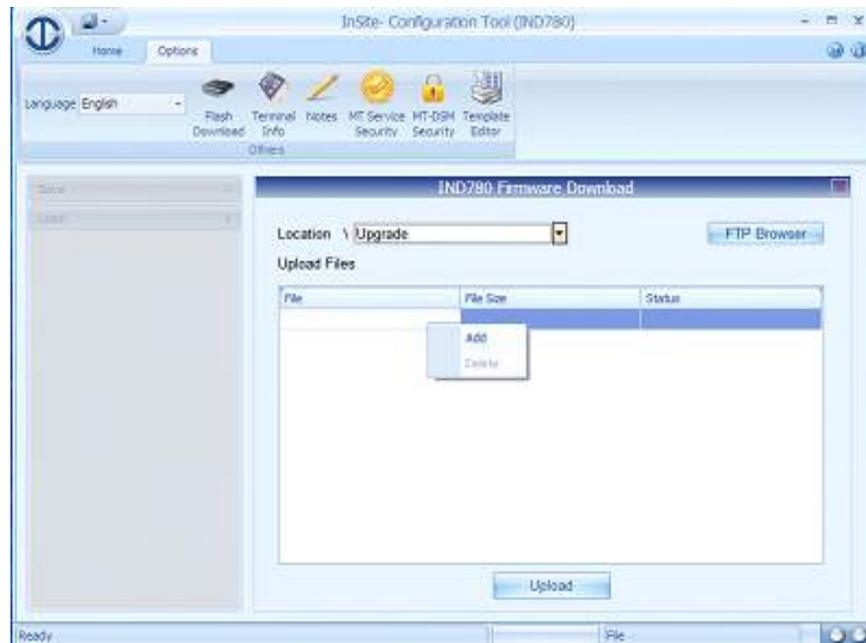
**Figure 4-1: InSite Firmware Upgrade File Selection Screen**
