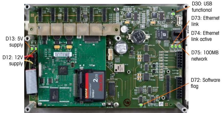
**Figure A-39: Main PCB LEDs**
