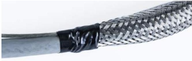
**Figure A-54: Outer Sheath Secured with Electrical tape**
