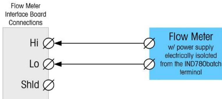
**Figure A-79: Isolated Flow Meter Connections**
