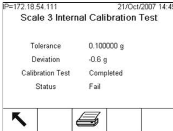
**Figure 3-188: Internal Calibration Test Complete Screen**
