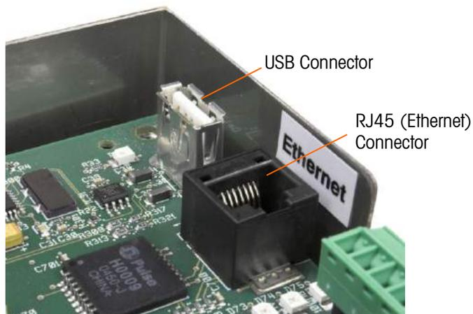
**Figure A-32: Ethernet and USB Connections**
