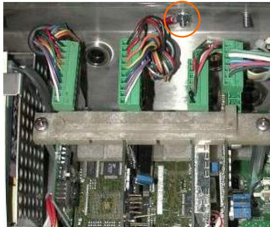
**Figure A-23: Shield Wire Termination, Harsh Enclosure**
