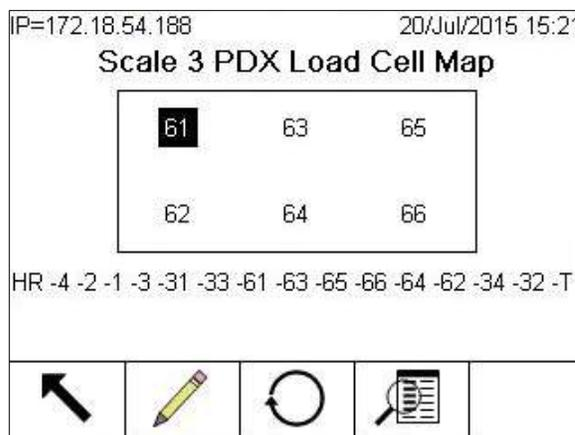
**Figure 3-176: Load Cell Map for Scale 3, All Cells Displayed**
