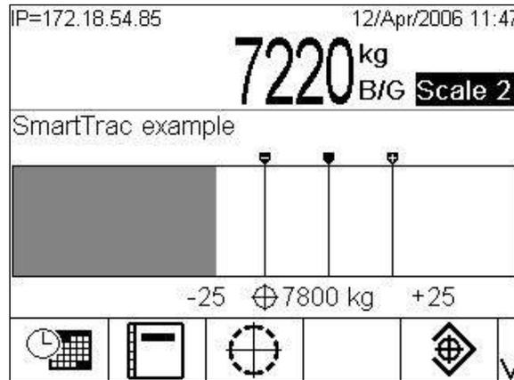
Figure 2-28: Bar Graph, Large SmartTrac Display
