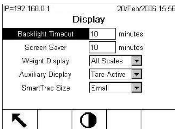
**Figure 3-96: Display Setup Screen**
