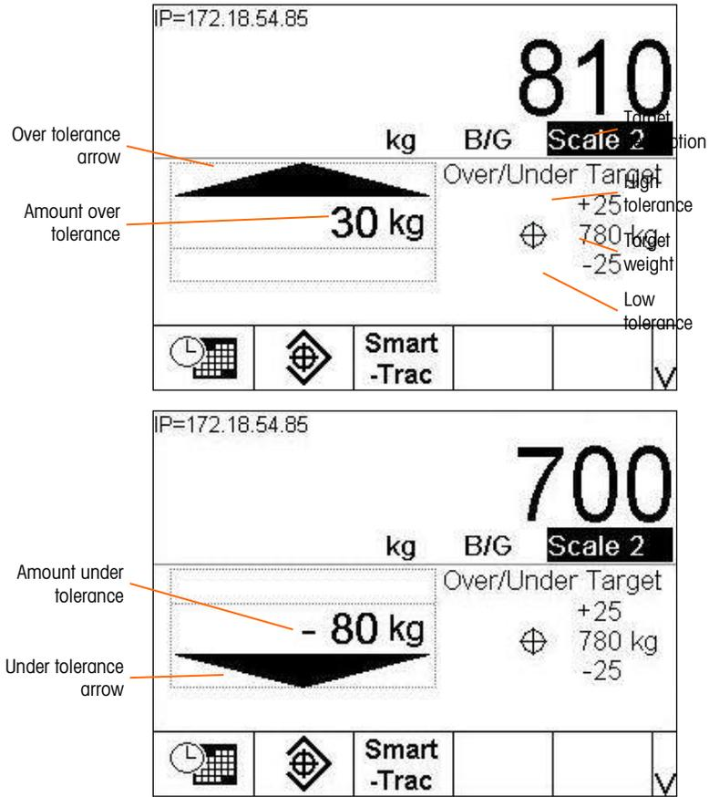
**Figure 2-31: Elements of the Over/Under SmartTrac Display**
