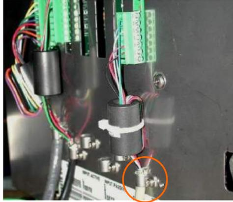
**Figure A-22: Shield Wire Termination, Panel Enclosure**
