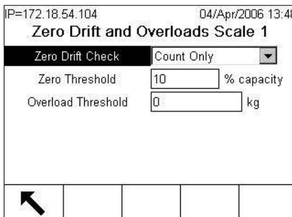
**Figure 3-161: Zero Drift and Overloads Screen**
