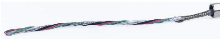
**Figure A-58: Inner Sheath Trimmed Back**
