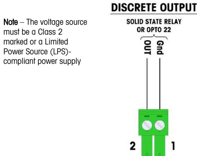
**Figure A-44: Analog Load Cell Discrete Output Connector**
