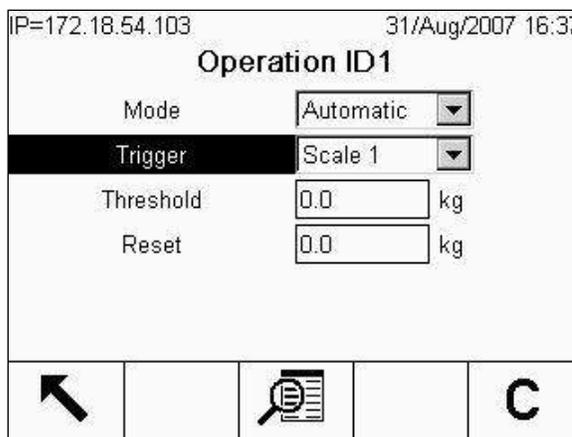
**Figure 3-84: ID1 Configuration Screen, Automatic Mode Selected**
