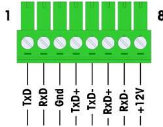
Figure A-35: COM2 Port Connections
