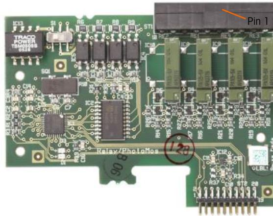
**Figure A-83: Discrete I/O Board, Relay**
