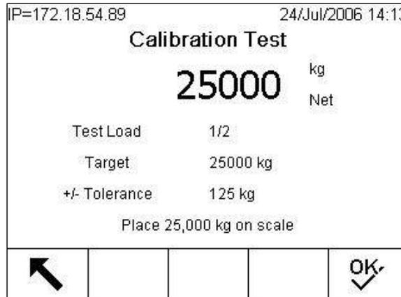
**Figure 3-182: Calibration Test Screen**
