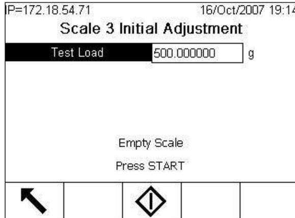
**Figure 3-40: Initial Adjustment Screen**
