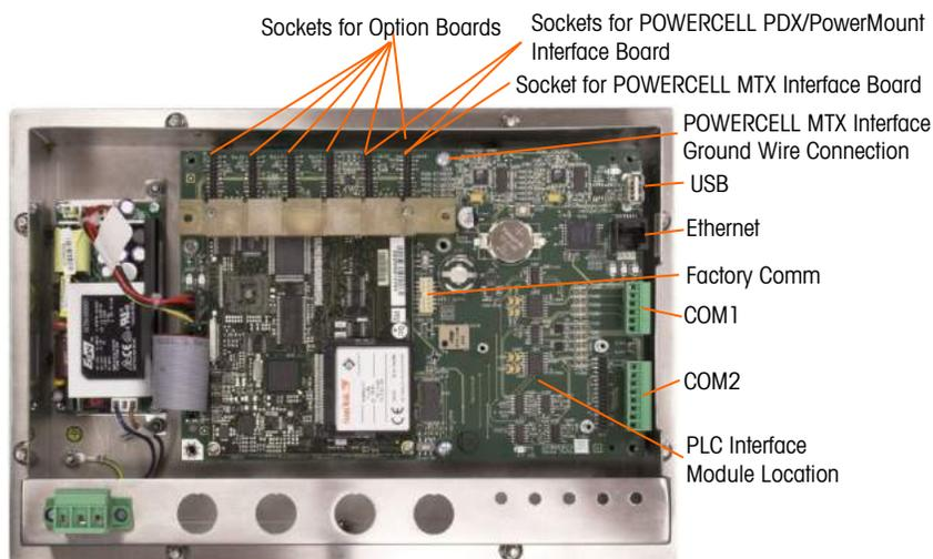
**Figure A-30: Wiring Connections, Top View, Panel Mount Enclosure**
