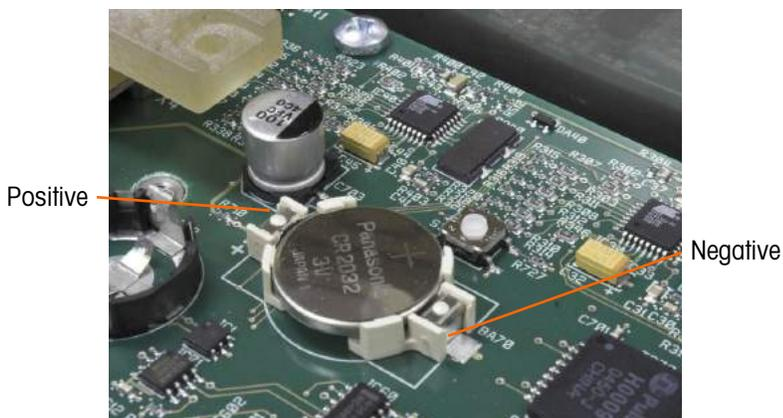
**Figure 4-16: Battery Installed**
