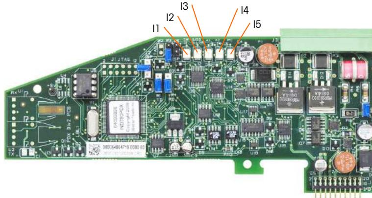
**Figure A-74: POWERCELL PDX Board LEDs**
