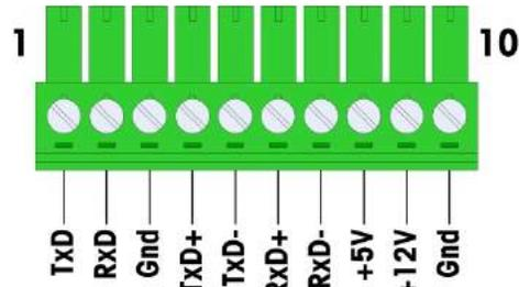
Figure A-92: Serial Option Board Connector
