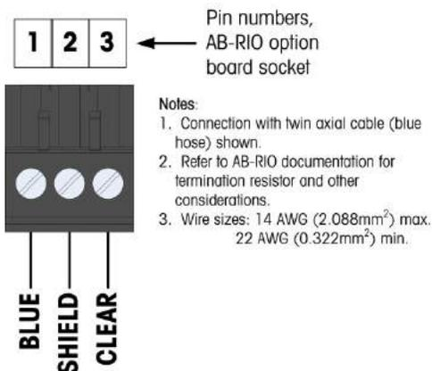
**Figure A-97: RIO Connection Wiring**
