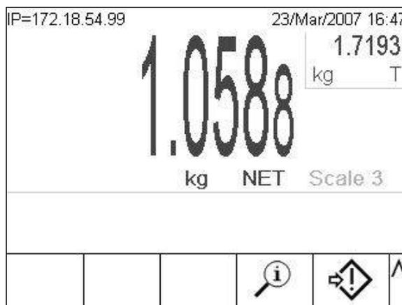
**Figure 2-17: Class II-Approved IDNet Base Weight Display**
