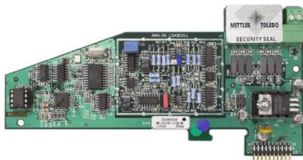
**Figure A-115: Security Seal Installed**
