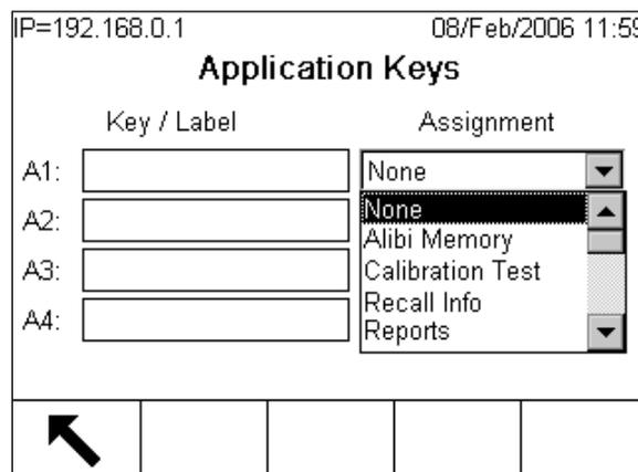
Figure E-7: Application Keys Setup Screen
