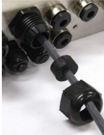
**Figure A-26: Cable Inserted Through Grommet, Nut, and Cable Grip**
