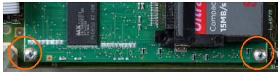
**Figure 4-56: ETX Board Mounting Screws**
