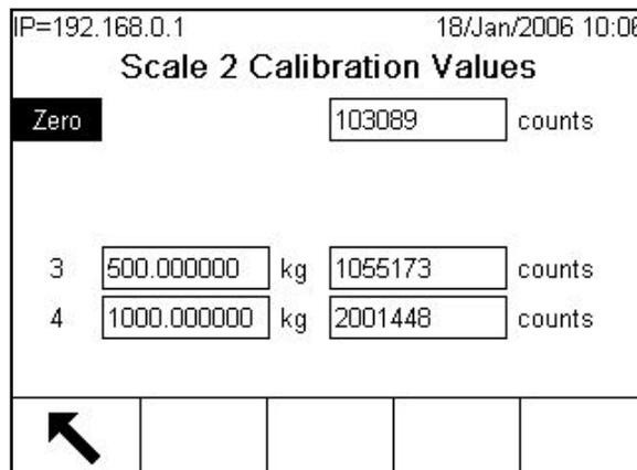
**Figure 4-22: Calibration Values Screen, Zero in Focus**
