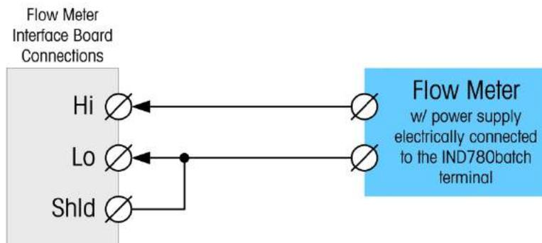
**Figure A-80: Non-Isolated Flow Meter Connections**
