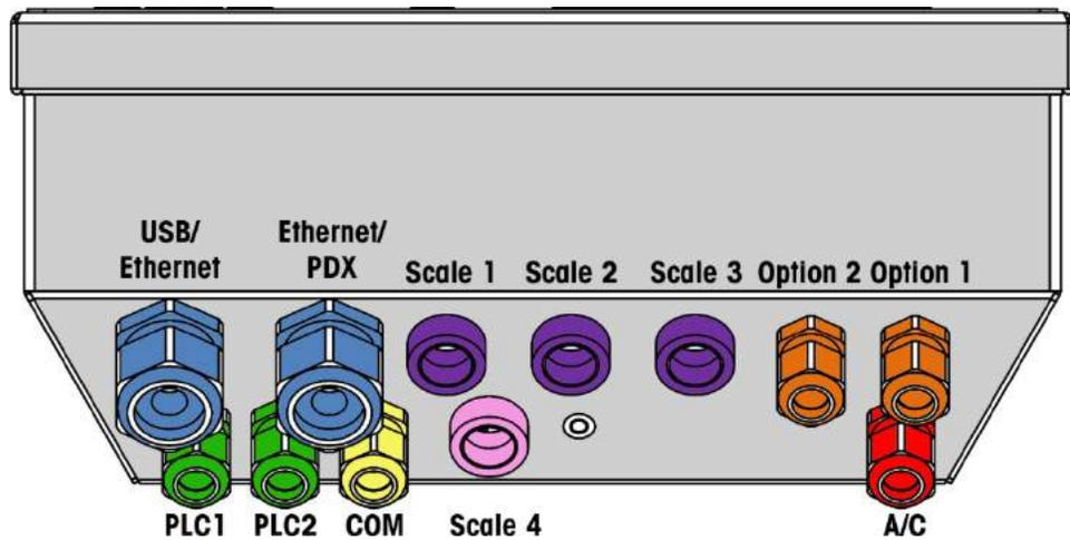
Figure A-24: Harsh Enclosure Cable Opening Assignments
