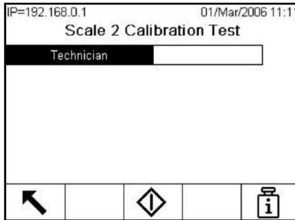
Figure 2-39: Calibration Test Name-Entry Screen
