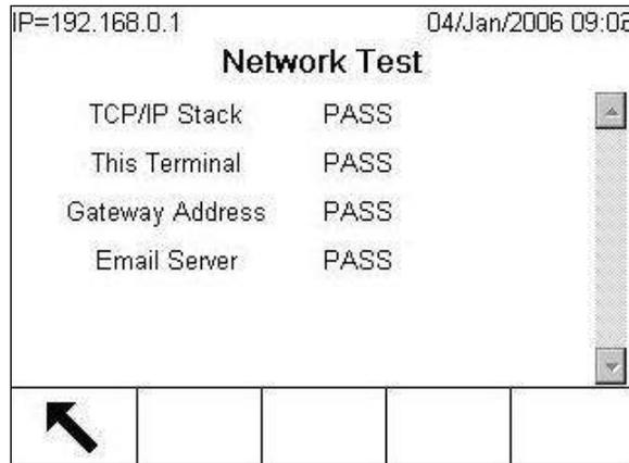
Figure 3-211: Network Test
