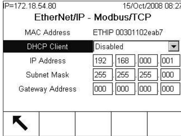
**Figure 3-141: EtherNet / IP PLC Interface Setup Screen**
