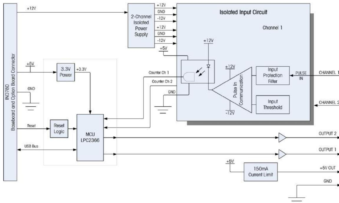
**Figure A-77: Block Diagram, Channel 1 Shown**
