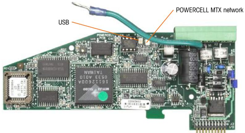
**Figure A-49: POWERCELL MTX LEDs**
