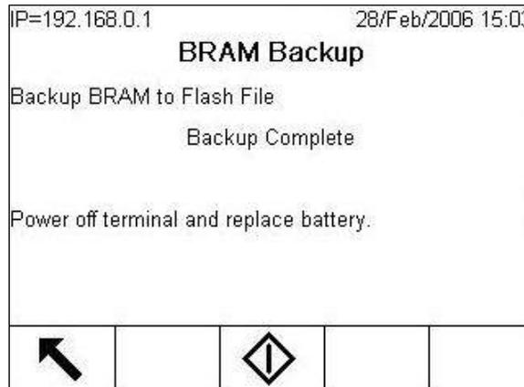
**Figure 3-213: Replace Battery Screen**
