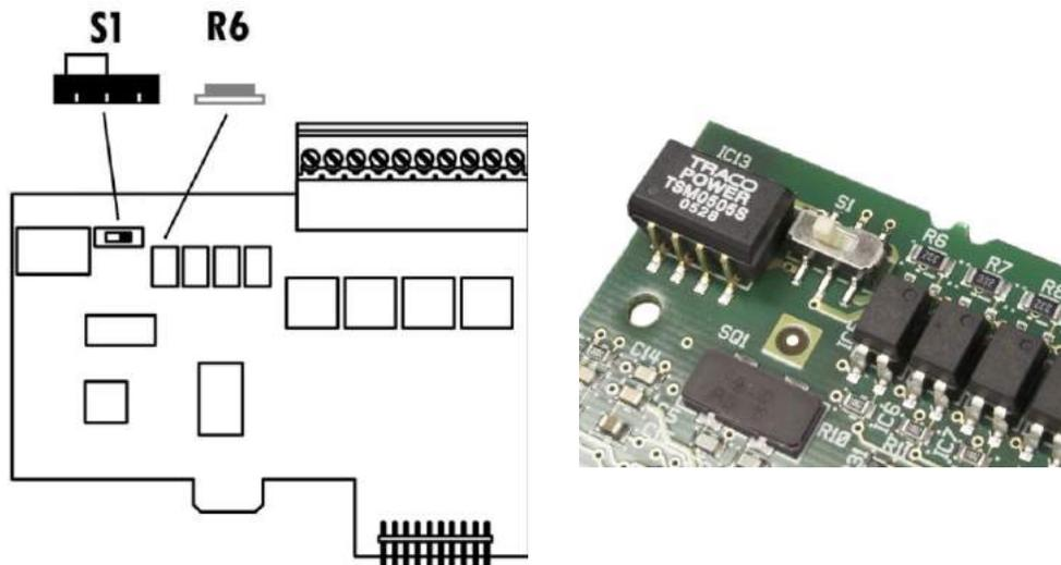
**Figure A-81: Discrete I/O Board Mode Selector Switch Location**
