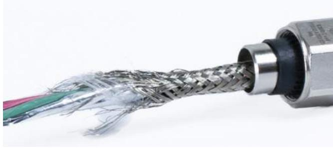
**Figure A-59: Inner Sheath Frayed**
