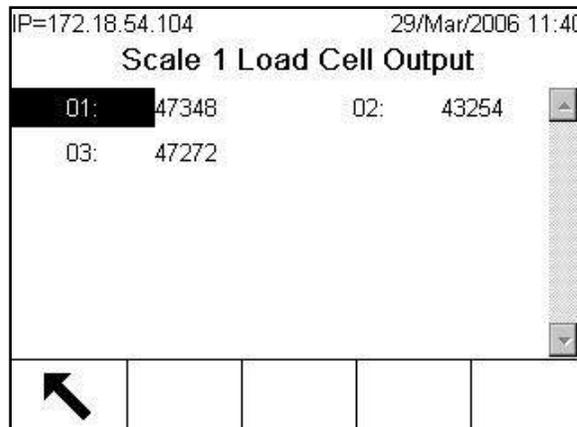
**Figure 4-21: Load Cell Output Screen**
