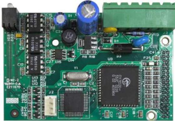
**Figure A-102: DeviceNet Option Board**
