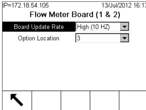
**Figure 3-63: Flow Meter Board Settings Screen**
