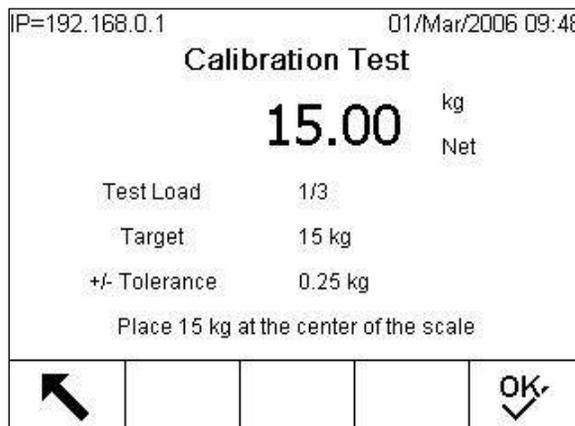
**Figure 2-41: Calibration Test Step**
