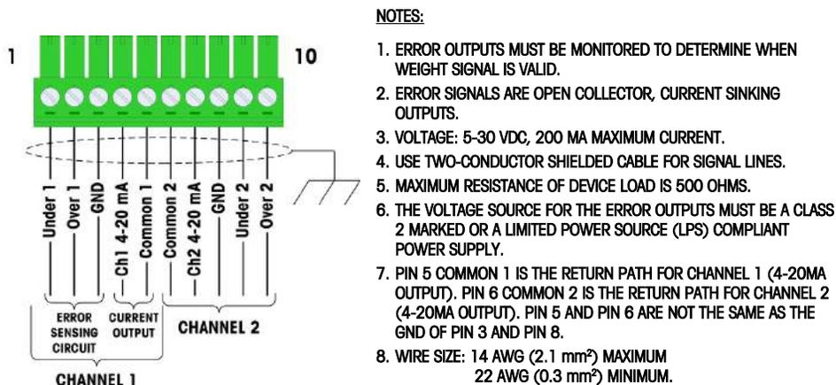
**Figure A-95: Analog Output Kit Wiring Connections**
