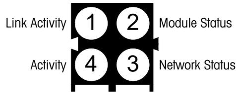
**Figure A-106: Ethernet / IP Status Indicator LEDs**
