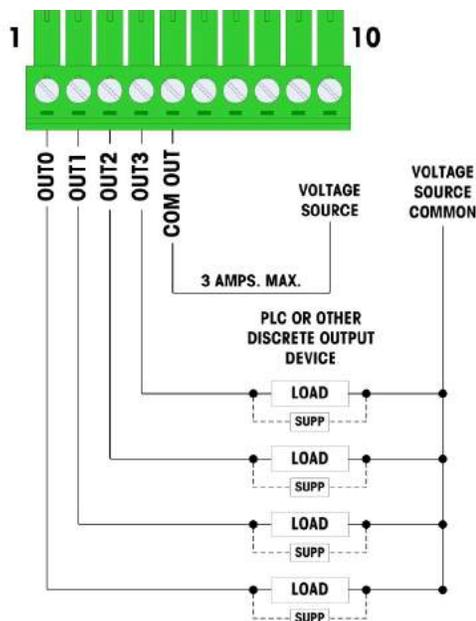
**Note** – The voltage source must be a Class 2 marked or a Limited Power Source (LPS)-compliant power supply.
