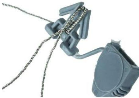
**Figure A-118: Wire Looped Around Seal**
