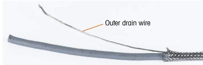
**Figure A-53: Outer Sheath Trimmed**
