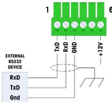
Figure A-34: COM1 Wiring for RS232
