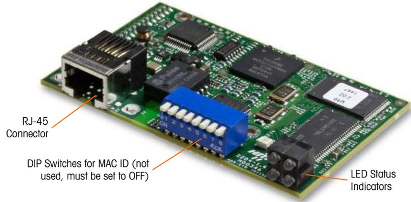
**Figure A-105: Ethernet / IP PLC Module Components**
