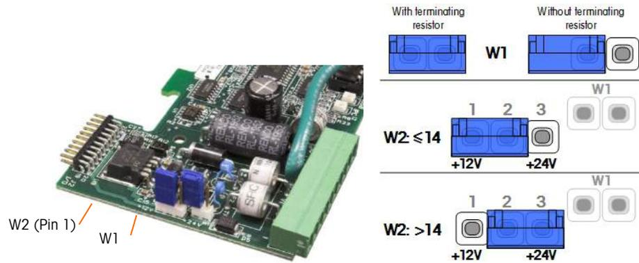
**Figure A-47: POWERCELL MTX Card Jumper Locations and Settings**
