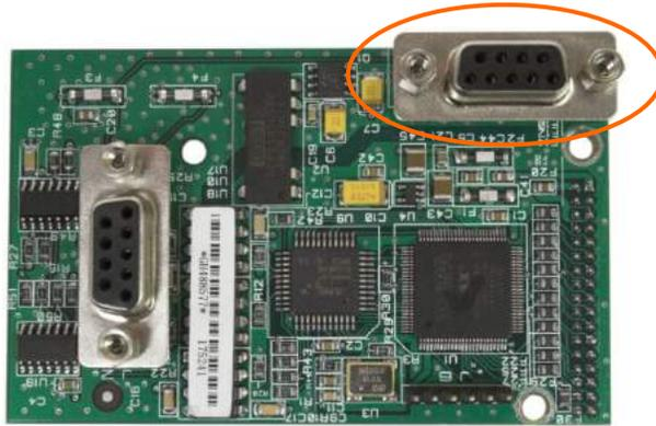
**Figure A-109: PROFIBUS PLC Module for Panel Mount Enclosure**
