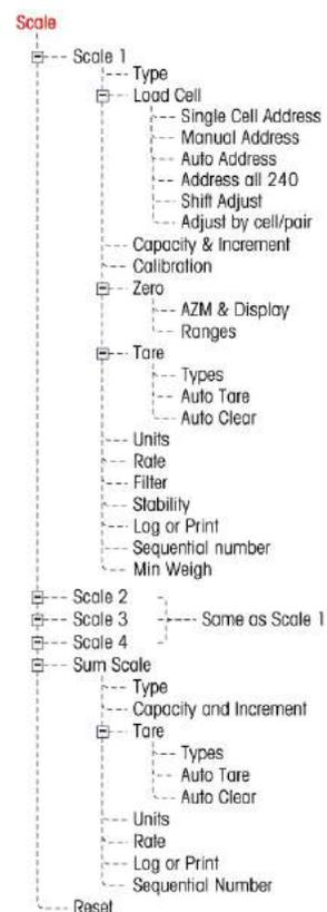
A Reset is present at the end of the branch to enable a limited reset to the factory default settings for the Scale parameters.
