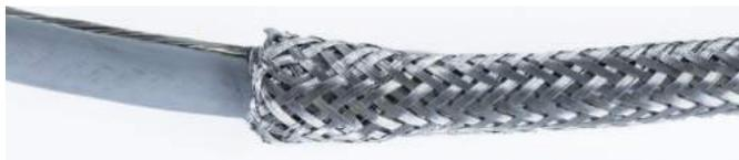
**Figure A-55: Outer Sheath Pushed Up Over Taped End**
