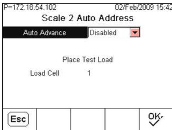
**Figure 3-21: Auto Address Place Load Screen, PDX**
