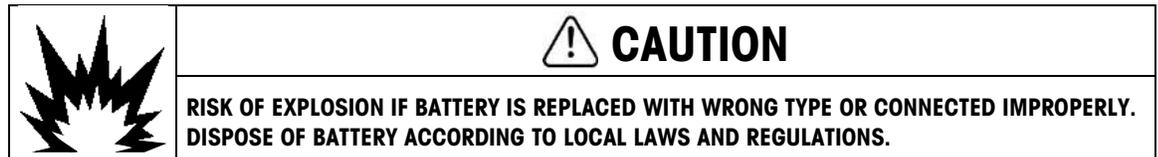
Changing the battery on the main PCB will cause volatile BRAM memory to be lost. Selecting Replace Battery opens a screen (Figure 3-212) prompting for BRAM Backup. This procedure should be performed during initial installation. Backing up the BRAM to flash also sets the clock used by the battery replacement monitor.
