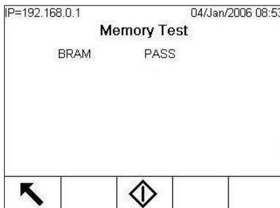
**Figure 4-18: Memory Test Screen**
