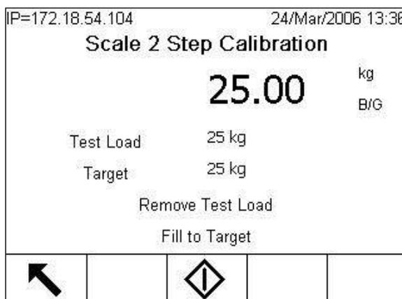
**Figure 3-32: Step Calibration, First Step Complete**
