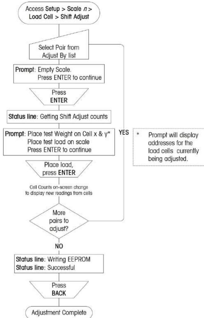
**Figure 3-22: Procedure for adjusting cells by pairs**
