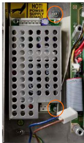
**Figure 4-63: Power Supply, Disconnected**
