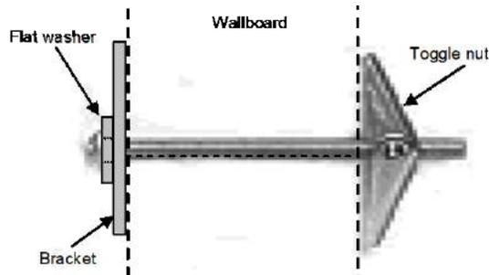
**Figure A-17: Wallboard or Drywall Installation**
