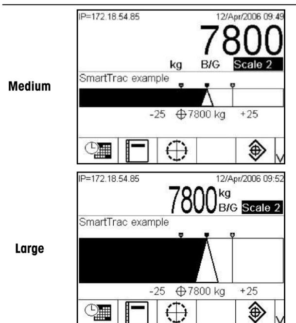
**Figure 3-97: Examples of Different Sizes of SmartTrac Displays**
