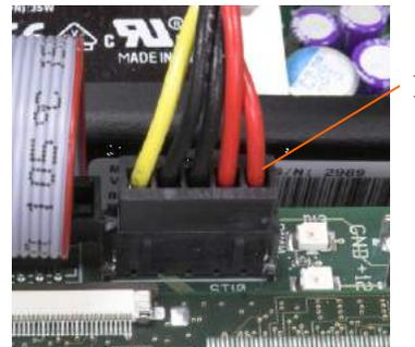
**Figure 4-14: Pins on the Power Supply Harness**
