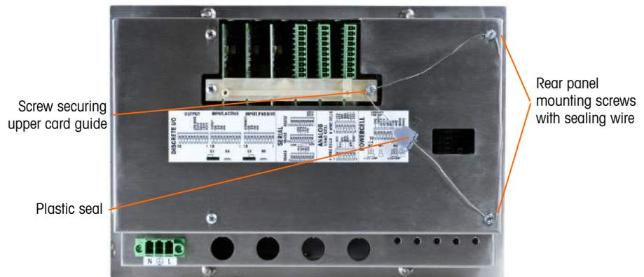
**Figure A-119: 3-Point Sealing, Panel Enclosure Rear Cover**
