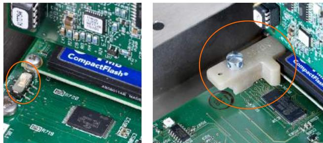
**Figure A-113: Metrology Security Switch (left) and Cover Installed (right)**
