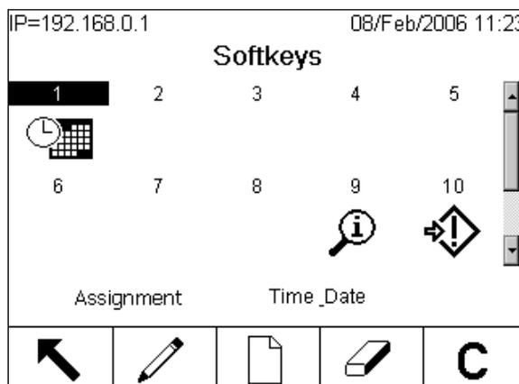
Figure E-3: Softkeys Setup Screen
