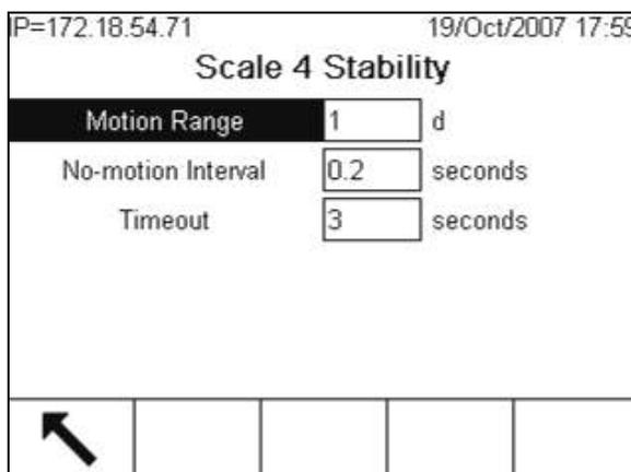
**Figure 3-55: Stability Setup Screen**
