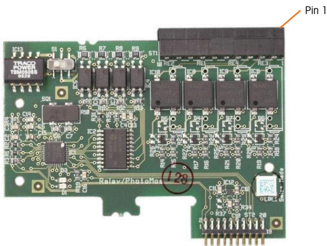
**Figure A-82: Discrete I/O Board, Solid State Relay**
