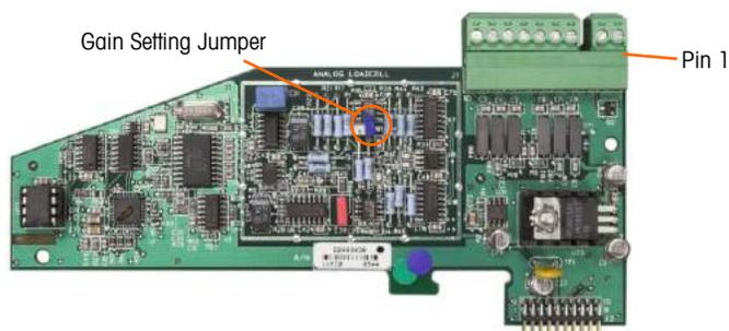
**Figure A-41: Analog Load Cell Option Board**
