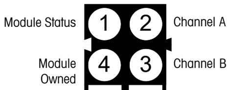
**Figure A-100: ControlNet Status Indicator LEDs**
