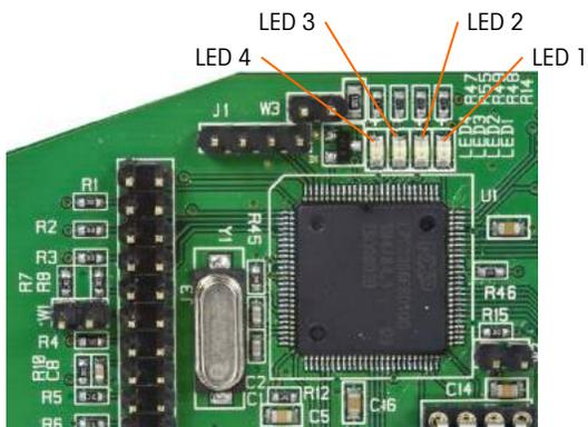
**Figure A-96: Analog Output LEDs**
