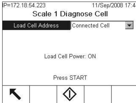
**Figure 3-204: Diagnose Cell Start Screen**
