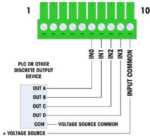
**Figure A-86: Example of Passive Input from Discrete Output Device**
