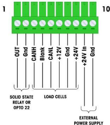
**Figure A-52: POWERCELL PDX Option Board Connections**
