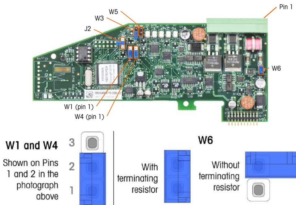
**Figure A-50: POWERCELL PDX Board Jumper Locations and Settings**
