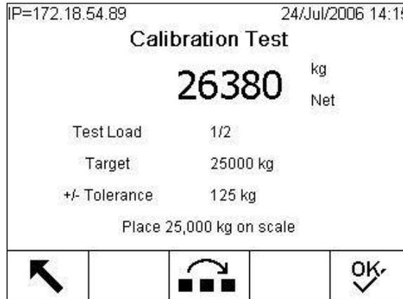
**Figure 3-184: Calibration Test Screen**
