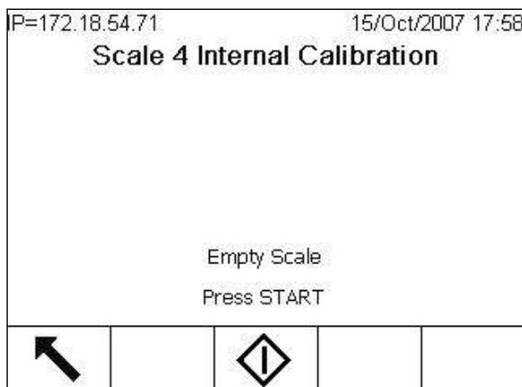
**Figure 3-34: Internal Calibration Screen**
