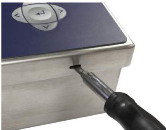
**Figure A-4: Opening the Harsh Enclosure, Alternative Method**
