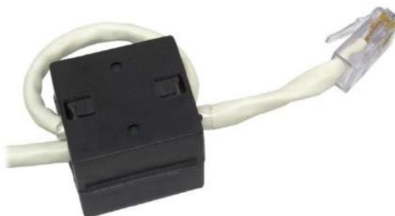
**Figure A-20: Installing Clamp Ferrite**
