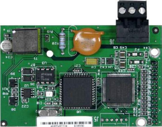
**Figure A-98: Allen Bradley RIO PLC Interface Module**
