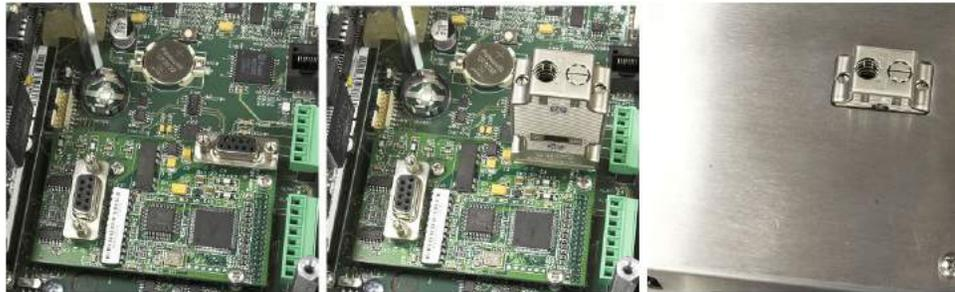
**Figure A-110: PROFIBUS PLC Module Connector for Panel Mount Enclosure**
