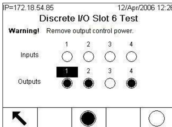
**Figure 4-29: Discrete I/O Test Screen**
