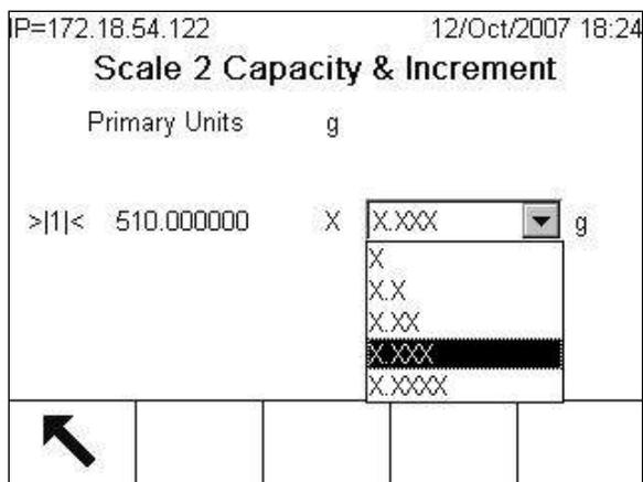
**Figure 3-25: Capacity and Increment Setup Screen, SICS**
