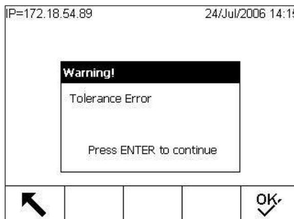
**Figure 3-183: Calibration Test Tolerance Error Screen**
