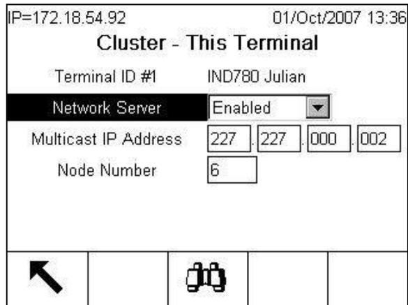
**Figure 3-128: Cluster – This Terminal Setup Screen**
