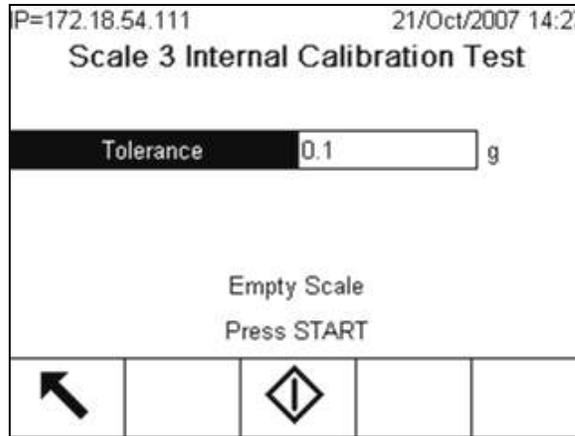
**Figure 3-186: Internal Calibration Test Screen**
