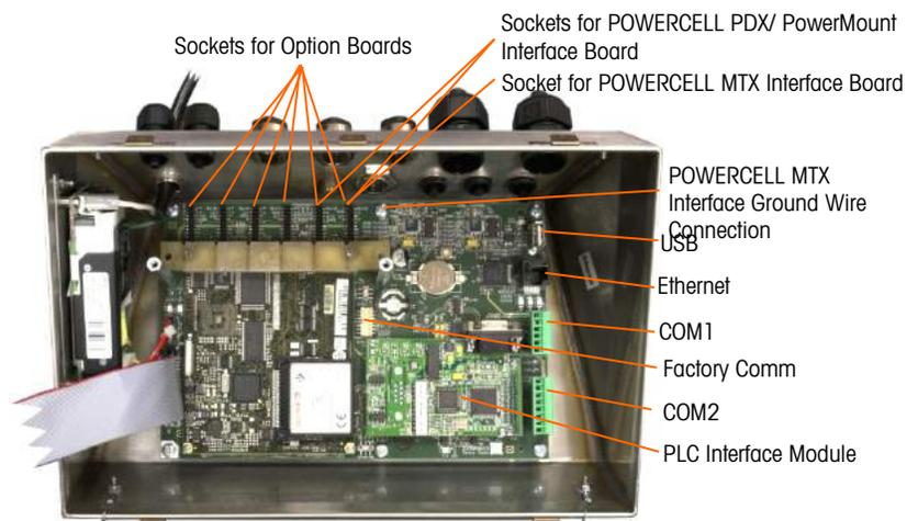
**Figure A-29: Wiring Connections, Top View, Harsh Enclosure**
