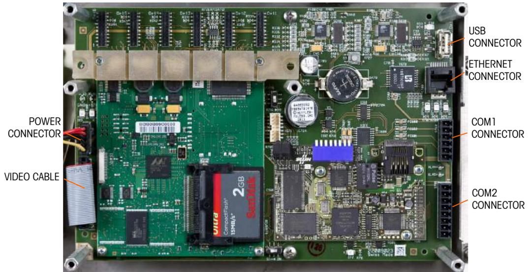
**Figure 4-13: Main PCB Connections and Mounting Screws**
