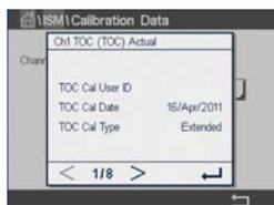
To view any of these calibration records, select the channel associated with the applicable 5000TOCi, the calibration, and the parameter to be reviewed from the drop-down selectors provided, then press the Cal Data button. Use the < and > icons to change pages to view the entire calibration record. Once viewing of the record is completed, press the ↩ icon to return to the Calibration Data screen.
