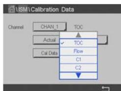
The 5000TOCi will store up to 4 sets of calibration data including the factory calibration (Factory), the current active calibration (Actual), and up to two of the most recent previous calibrations (Cal1 and Cal2, with Cal1 being the most recent historical calibration record). Each of these calibration records can be viewed from the M800.
