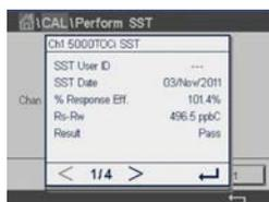
The 5000TOCi will store up to 4 sets of System Suitability Test results labeled SST-1 (most recent) through SST-4. The results of each of these SST procedures can be retrieved through the M800 transmitter.
