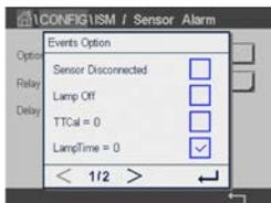
The ISM / Sensor Alarm feature allows configuring an alarm relay to provide an external indication of selected alarm conditions. When any of the selected events occur, a Flashing Red Bar will be displayed on the M800, and the alarm relay will energize if configured.
