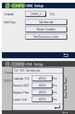
Calibrate TOC: Define the maximum time period in hours before a calibration must be performed.
