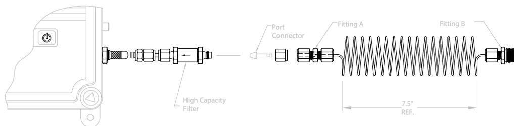
1. Remove compression fitting from filter assembly. As shown, insert port connector into compression fitting that was removed from filter. Reconnect compression fitting to the filter assembly and tighten to crimp. Do not over tighten.
