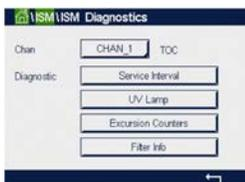
The ISM Diagnostics menu allows viewing many characteristics of the 5000TOCi to allow assessing the general condition of the sensor.
