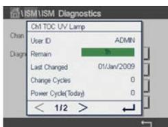
setting under ISM Setup. This value is reset to the Lamp Limit setting when a lamp replacement is registered through the TOC Maintenance menu.
