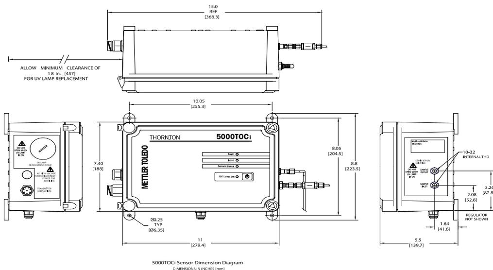
Shown above are the case dimensions for the 5000TOCi Sensor. Mount the 5000TOCi Sensor as close to the sample point of your system as possible. Shorter sample tubing length between the sampling point and the 5000TOCi Sensor will provide a faster response time. As shown above, the 5000TOCi Sensor is supplied with wall-mounting tabs for wall or panel mount.
