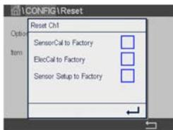
The M800 provides the ability to reset various settings within connected sensors to factory default values. To reset parameters associated with the 6000TOCi, enter the Reset menu and select the channel associated with the 6000TOCi to be reset from the drop-down selector provided. To configure the reset function, press the 'Configure' button, select the specific parameter sets that are to be reset to the factory values, and press the **←** icon.
