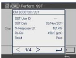
The 6000TOCi will store up to 10 sets of System Suitability Test results labeled SST-1 (most recent) through SST-10. The results of each of these SST procedures can be retrieved through the M800 transmitter.
