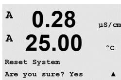
Pressing the [ENTER] key after the selection will bring up a confirmation screen. Selecting No will return the user to the Measurement mode with no changes. Selecting Yes will reset the meter.
