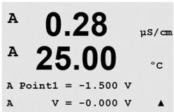
Enter the value for Point 2, in volts, of the source connected to the input. The second display line shows the measured voltage.
