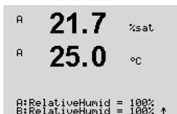
In addition the relative humidity of the calibration gas can also be entered. The allowed values for relative humidity are in the range 0% to 100%.
