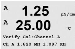
Use the ▲ or ▼ key to toggle between Channel A and B\*.
