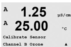
Enter Ozone Calibration mode as described in section 7.1 "Enter Calibration Mode" and select Ozone.
