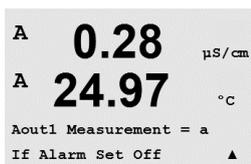
When an Alarm Value is selected, the analog output will go to this value if any alarm condition occurs.
