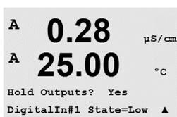
The "DigitalIn" function applies all the time. As soon as a signal is active on the digital input the transmitter goes to hold mode and the values on the analog output, the output relays and the USB output will be at hold state.
