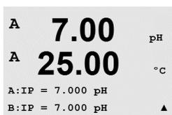
IP is the isothermal point value (Default = 7.000 for most applications). For specific compensation requirements or non standard inner buffer value, this value can be changed. Press [ENTER].
