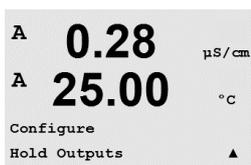
The "Hold outputs" function applies during the calibration process. If set "Hold outputs" to Yes, during calibration process the analog output, the output relay and USB output will be at hold state. The hold state depends on the setting. For the possible hold settings, see the list below. The following options are possible:
