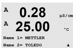
Use the ◀ and ▶ keys to navigate between digits to be altered. Using the ▲ and ▼ keys to change the character to be displayed. Once all digits of both display channels have been entered, press [ENTER] to bring up the Save Changes dialog.
