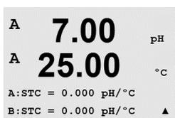
STC is the solution temperature coefficient in units of pH/°C referenced to 25 °C (Default = 0.000 for most applications). For pure waters, a setting of –0.016 pH/°C should be used. For low conductivity power plant samples near 9 pH, a setting of –0.033 pH/°C should be used. These negative coefficients compensate for the negative temperature influence on the pH of these samples. Press [ENTER].
