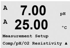
For dual channel devices: The menu Comp/pH/O2 can be selected by using the ▲ or ▼ key. Then use the ► key to move to the next input field and select the parameter using the ▲ or ▼ key. The choices are Resistivity (for conductivity measurement), pH and O2. Press [ENTER]
