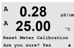
Pressing the [ENTER] key after the selection will bring up a confirmation screen. Selecting No will return the user to the Measurement mode with no changes. Selecting Yes will reset the meter calibration factors.
