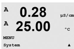
While in Measurement mode press the ◀ key. Press the ▼ or ▲ key to navigate to “System” – Menu and press [ENTER].
