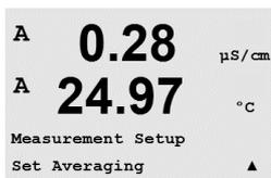
Press the [ENTER] key to select this Menu. The averaging method (noise filter) for each measurement line can now be selected. The options are Special (Default), None, Low, Medium and High:
