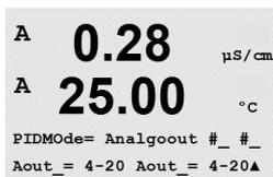
**Analog** – If using Analog control, change “Relays” to “Analogout” using up/down arrow keys. Choose the first Analogout position as #1 and/or the second Analogout position as #2 according to the table below. Select the analog output current range required by the control device, 4–20 or 0–20 mA. Press [ENTER].
