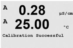
The transmitter will return to the Measurement mode in approximately 5 seconds.
