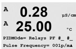
**Pulse Frequency** – If using a pulse input metering pump, select “Relays” and “PF”, Pulse Frequency. Choose the first relay position as #3 and/or the second relay position as #4 according to the table below. Set the pulse frequency to the maximum frequency allowed for the particular pump being used, typically 60 to 100 pulses/minute. Control action will produce this frequency at 100% output.
