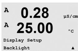
Possible settings are On, On 50% or Auto Off 50%. If Auto Off 50% is selected then the backlight will go to 50% after 4 minutes with no keypad activity. The backlight will automatically come back on if a key is pressed.
