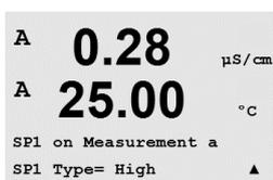
4 (6 for dual channel version) Setpoints can be configured on any of the measurements (a thru d). The possible Setpoint types are Off, High, Low, Outside and Between. Thornton models also include types, %USP, %EP PW and %EP WFI for configuration with conductivity sensors.
