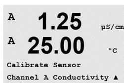
While in Measurement mode press the ► key. If the display prompts you to enter the calibration security code, press the ▲ or ▼ key to set the calibration security mode, then press the [ENTER] key to confirm the calibration security code.
