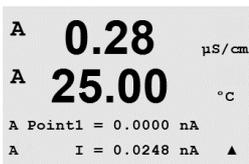
Enter the value for Point 2, in milliamps, of the current source connected to the input. The second display line shows the measured current.
