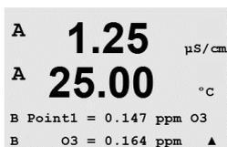
After the calibration the slope calibration factor S and the offset calibration factor Z are displayed.
