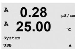
This menu allows configuration of the USB hold function.
