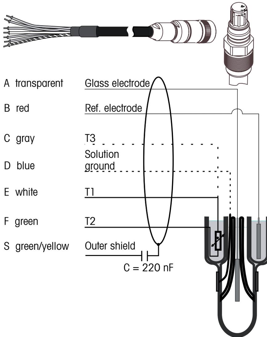
T1/T2: Temperature probe for 2-wire connection
