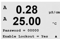
The Lockout – Menu is protected: Enter the Administrator Password and select YES to enable or NO to disable the Lockout functionality. Pressing the [ENTER] key after the selection will bring up the Save Changes dialog. Selecting No will discard the entered value, selecting Yes will make the entered value the current one.
