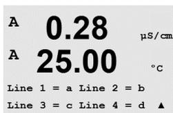
Select the "Error Display" mode. If this is set to "On" when an alarm has occurred, the message "Failure – Press Enter" will be displayed on Line 4 when an alarm occurs in the normal Measurement mode.
