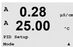
This menu contains the selection of control modes using relays or analog outputs. Press [ENTER].
