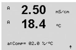
If compensation mode “Lin 25 °C” or “Lin 20 °C” has been chosen, the factor for the adjustment of the reading can be modified after pressing [ENTER] (If working at measurement line a or b press [ENTER] twice).
