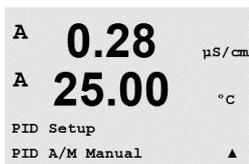
This menu allows selection of Automatic or Manual operation. Select Auto or Manual operation. Pressing the [ENTER] key will bring up the Save Changes dialog.
