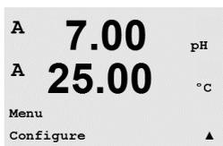
While in Measurement mode, press the ◀ key. Press the ▲ or ▼ key to navigate to the Configure – Menu and press [ENTER].
