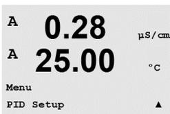
While in Measurement mode press the ◀ key. Press the ▲ or ▼ key to navigate to the PID Setup – Menu and press [ENTER].
