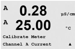
Enter the value for Point 1, in milliamps, of the current source connected to the input. The second display line will show the measured current. Press
