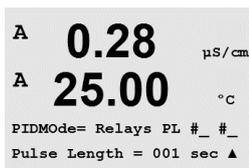
This menu assigns a relay or analog output for PID control action as well as details of their operation. Based on the control device being used, select one of the following three paragraphs for use with solenoid valve, pulse input metering pump or analog control.
