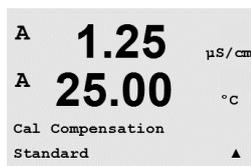
All other models provide the options "Standard", "Lin 20°C = 02.0%/°C" (user selectable value), and "Lin 25°C = 02.0%/°C" (user selectable value) as Compensation mode thru the calibration.
