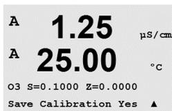
Select Yes to save the calibration values and the successful Calibration is confirmed on the display.
