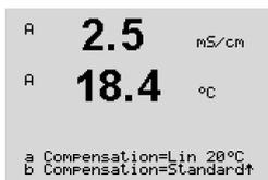
Lin 20 °C compensation adjusts the reading by a factor expressed as a “% per °C” (deviation from 20 °C). Use only if the solution has a well-characterized linear temperature coefficient. The factory default setting is 2.0%/°C.
