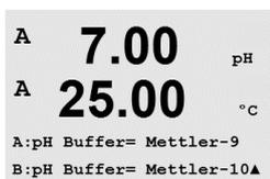
For automatic buffer recognition during calibration, select the buffer solution set that will be used: Mettler-9, Mettler-10, NIST Tech, NIST Std, HACH, CIBA, MERCK, WTW, JIS Z 8802 or None. See Section 20 “Buffer Tables” for buffer values. If the auto buffer feature will not be used or if the available buffers are different from those above, select None. Press [ENTER].
