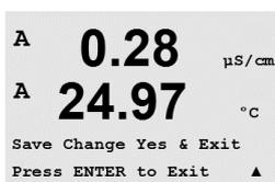
Pressing the [ENTER] key again will bring up the Save Changes dialog. Selecting No will discard the entered values and return to the measurement display screen, selecting Yes will save changes made.
