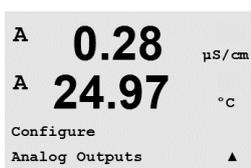
Enter configuration mode as described in Section 8.1 "Enter Configuration Mode" and navigate to the menu "Analog Outputs" by using the ▲ or ▼ key.
