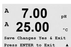
Selecting No will discard the entered values and return to the measurement display screen, selecting Yes will save changes made.
