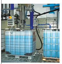
In many processes, integrated weighing sensors have been found to yield better results than flow meters, because weighing sensors do not require cleaning when your materials change.
