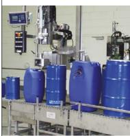
When your product is expensive, you shouldn't give it away through bulk container overfilling. METTLER TOLEDO load cells, weigh modules or scales can be easily integrated into your filling machine for accuracy in safe and hazardous environments, ensuring you deliver high fill accuracies to achieve cost savings.
