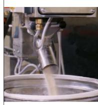
Dry materials are best processed by weighing, because weight is a more constant measurement than volume. If you are seeing variations in your weighing results, consider using METTLER TOLEDO automation sensors and METTLER TOLEDO load cells in your loss-in-weigh systems.
