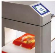
When foreign bodies in your product could harm customers, or following processes, consider an in-process metal detector or x-ray inspection system to automatically reject non-compliant products. This not only protects consumers — but also downstream production or packaging equipment against damage.
