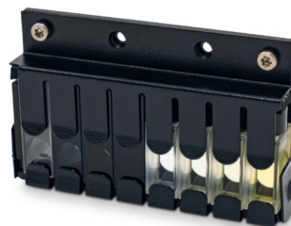
Inside LinSet Sealed liquid CRM cuvettes and solid certified neutral density filter
