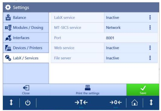
7 XPR/XSR Analytical Balance via USB: Tap LabX / Services and set the MT-SICS service value as USB.
