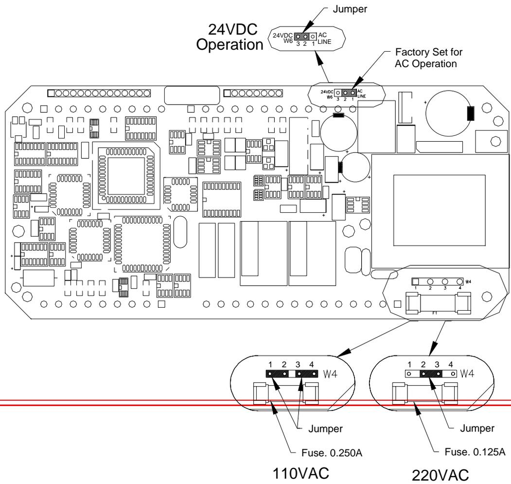
Figure 14.7: Printed Circuit Board Layout
