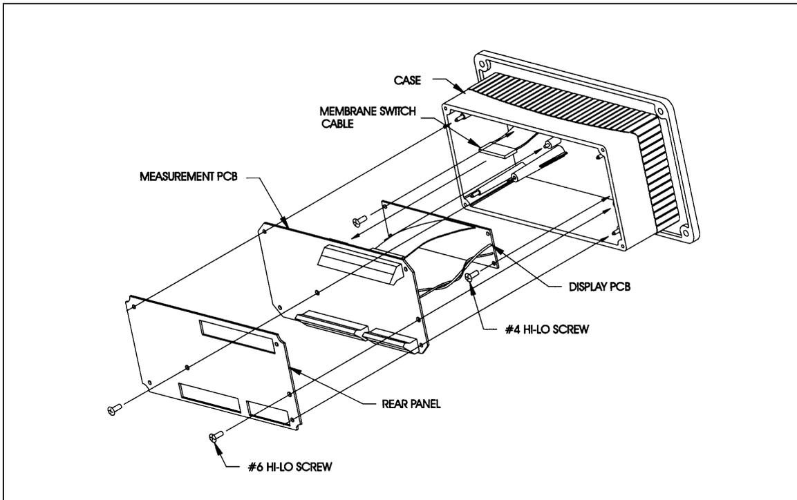
Figure 14.4: Exploded Assembly
