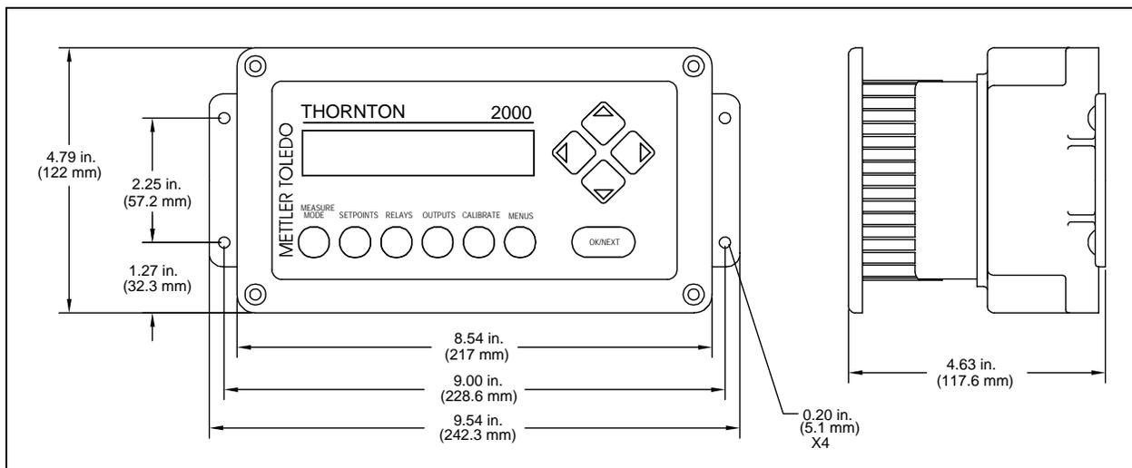
**Figure 14.2b: Wall Mounting Dimensions (with accessory back cover installed)**
