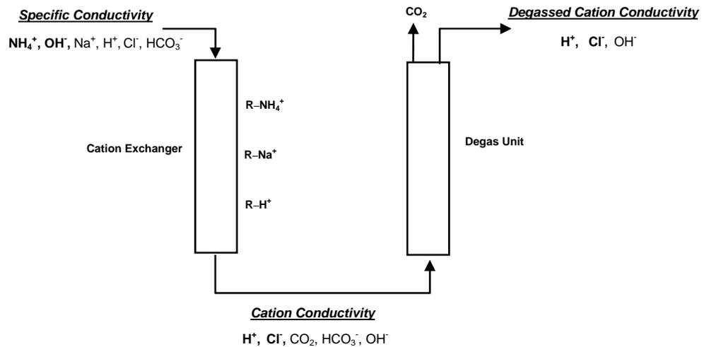
**Fig. 4.2: Sample conditioning for specific, cation and degassed cation conductivity measurements used to calculate pH, CO<sub>2</sub> and anion concentration on power plant cycle chemistry samples**
