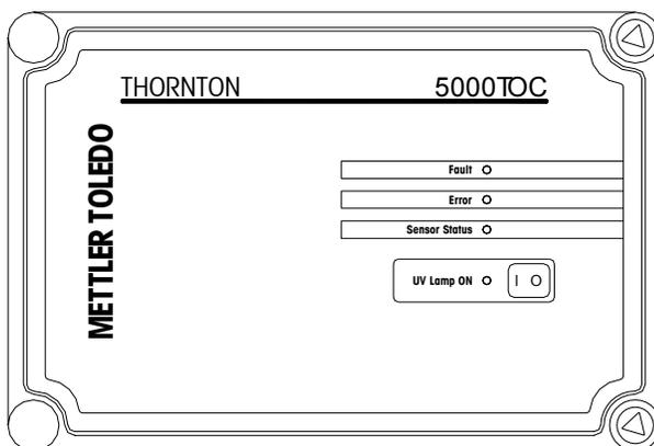
**Figure 4. 5000TOC Sensor Front Panel**
