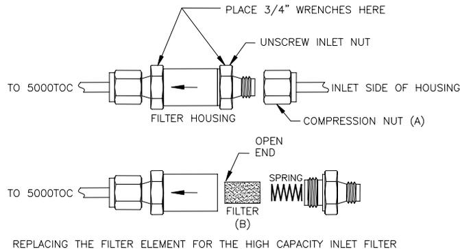
**Figure 7. High Capacity Inlet Filter Replacement**
