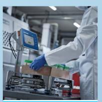
Multi-Zone Checkweighing Implement over/under checkweighing for 3 or 5 zones to improve net content control. The graphical multi-color zone alert visualization speeds up operation, and you can set zone tolerances in the local material table.
