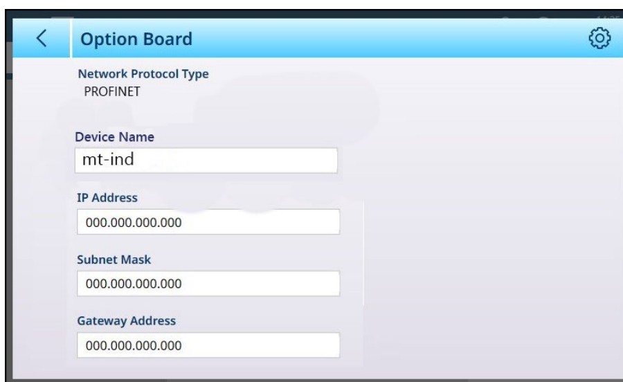
Figure 3-7: PROFINET Option Board Setup Menu
