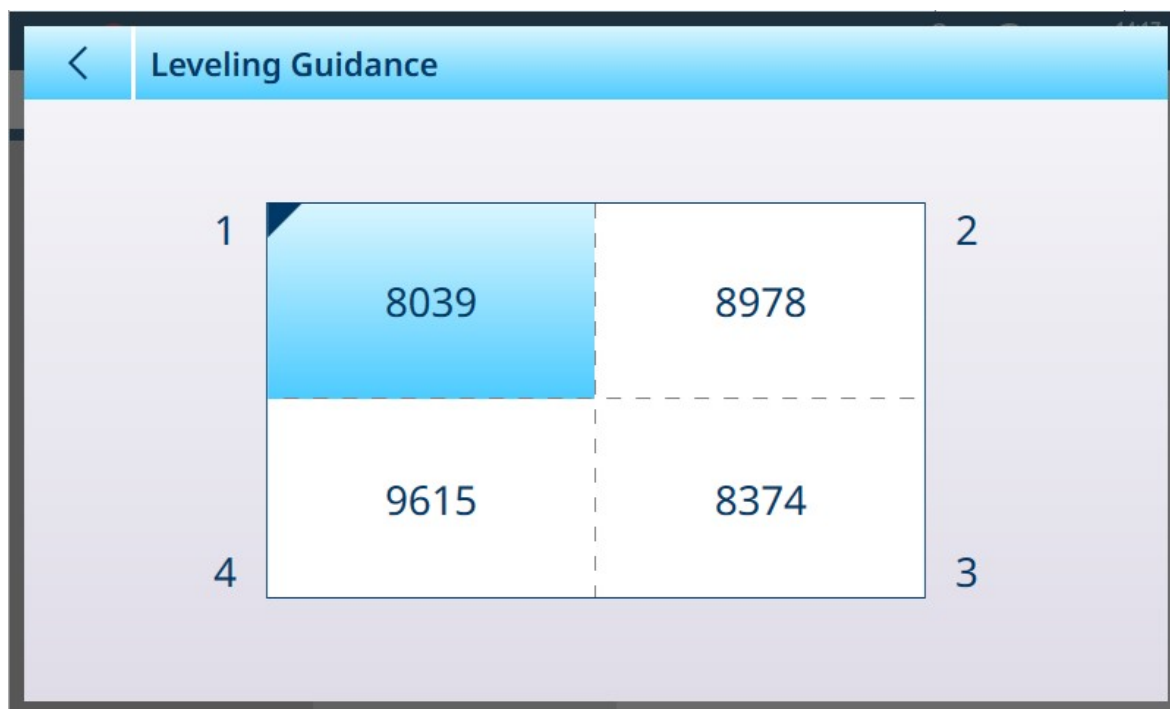
Figure 536: Leveling Guidance, 4 Load Cell Scale
