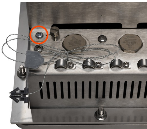
Figure 67: Sealing Screw Location, Panel Mount Enclosure
