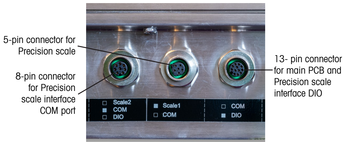
Figure 57: External M12 Connectors Associated with Precision Interface Board
