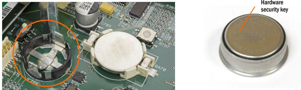
Figure 1-2: IND780 Hardware Key Socket on Mother Board
