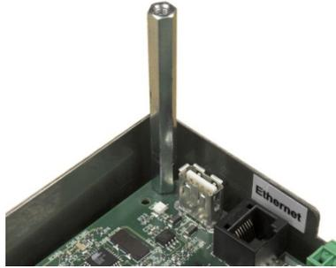
**Figure 4-49: Stand-Off on Main PCB**
