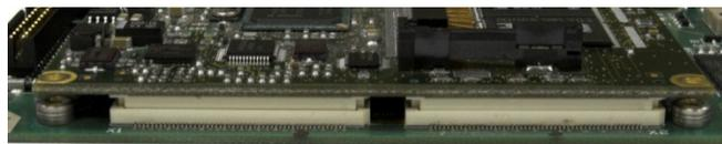
**Figure 4-54: ETX Board Resting on Connectors**
