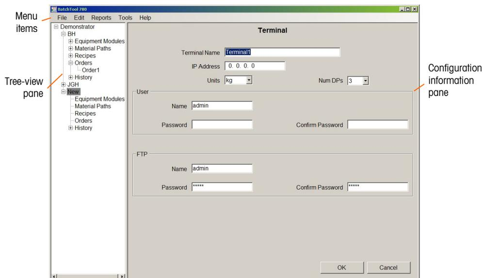
**Figure 6-1: PC Tool Interface Layout**
