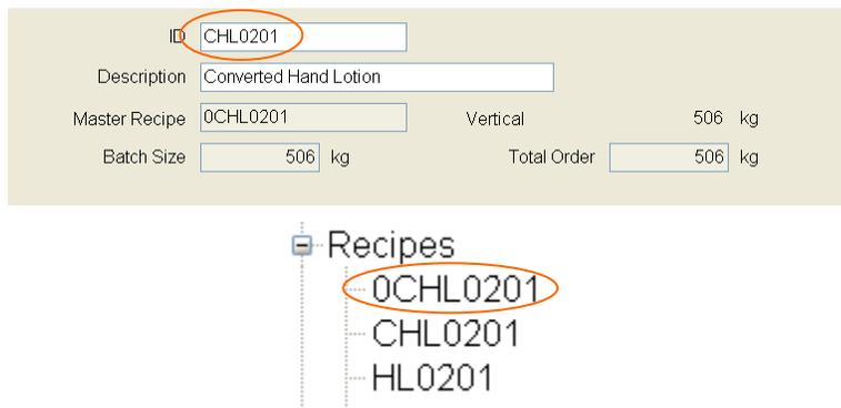
**Figure 12-8: Displays in BatchTool 780 and Terminal, Showing a Converted Batch**
