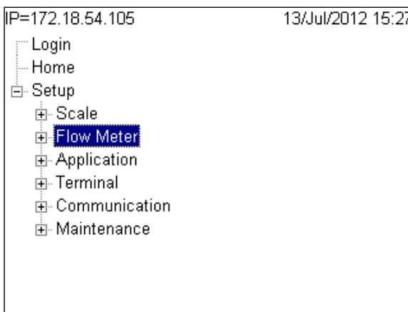
**Figure 3-31: Flow Meter Branch in Setup Menu Tree**
