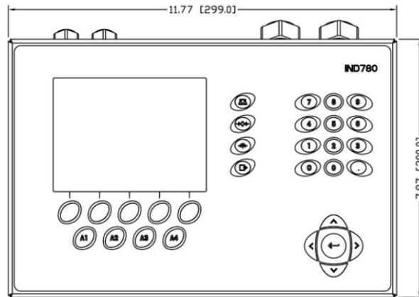
Figure 1-7: IND780batch Harsh Enclosure Terminal Dimensions, Front
