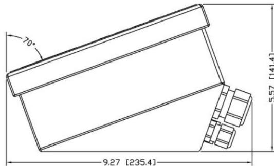
Figure 1-8: IND780batch Harsh Enclosure Terminal Dimensions, Side
