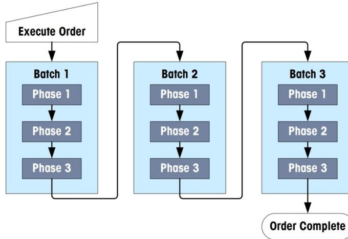
**Figure 2-3: Structure of a Vertical Campaign**
