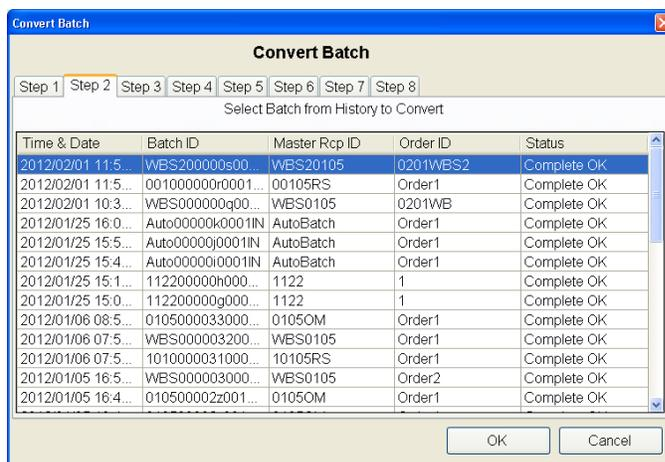
**Figure 12-25: Convert Batch Source Recipe Selection Screen**
