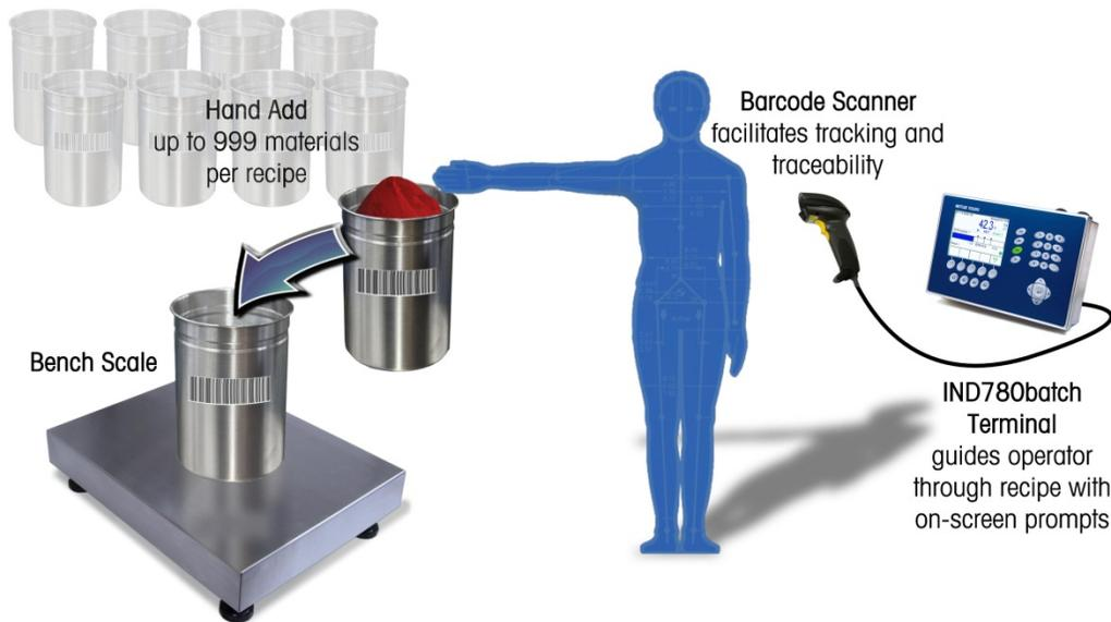
Figure 1-11: Manually Controlled Batching System
