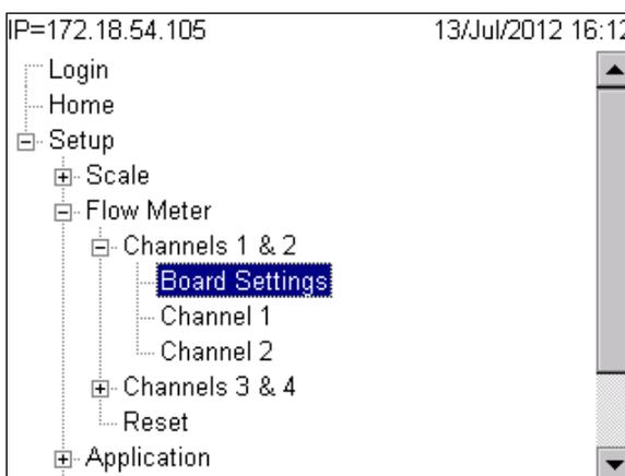
**Figure 3-32: Board Settings Branch in Flow Meter Setup Menu**
