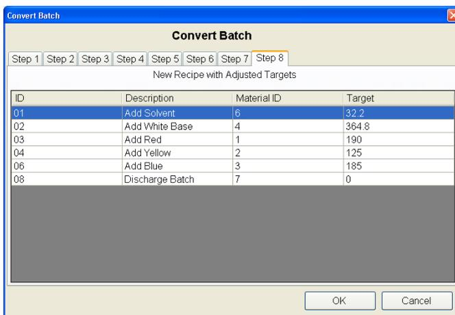
The screenshot shows the same "Convert Batch" dialog box as in Figure 12-26, but with the "Step 8" tab selected. The table content is identical to the one in Figure 12-26, showing the adjusted target amounts for each ingredient. The "OK" and "Cancel" buttons are visible at the bottom.
