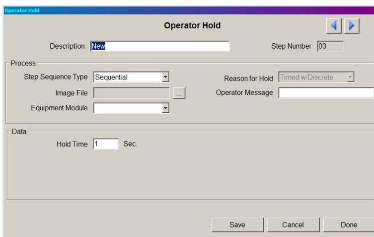
**Figure 11-18: Phase: Operator Hold, Timed with Discrete**
