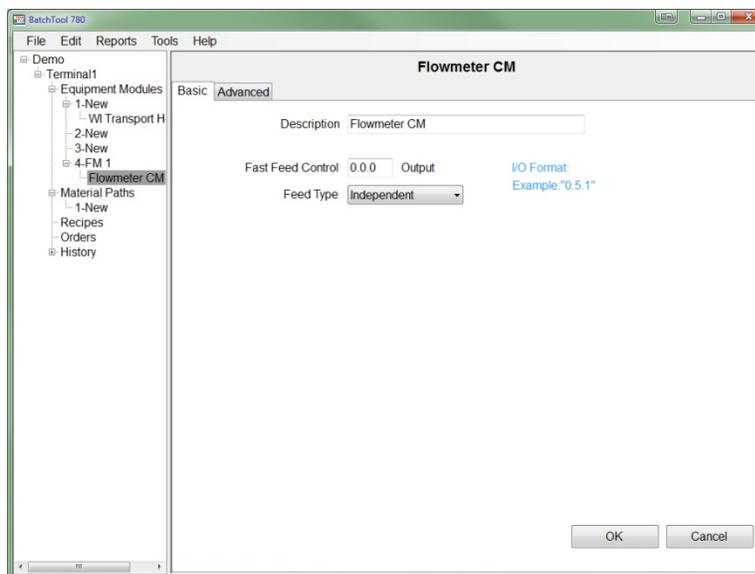
Figure 9-19: Flow Meter Control Module, Basic Tab
