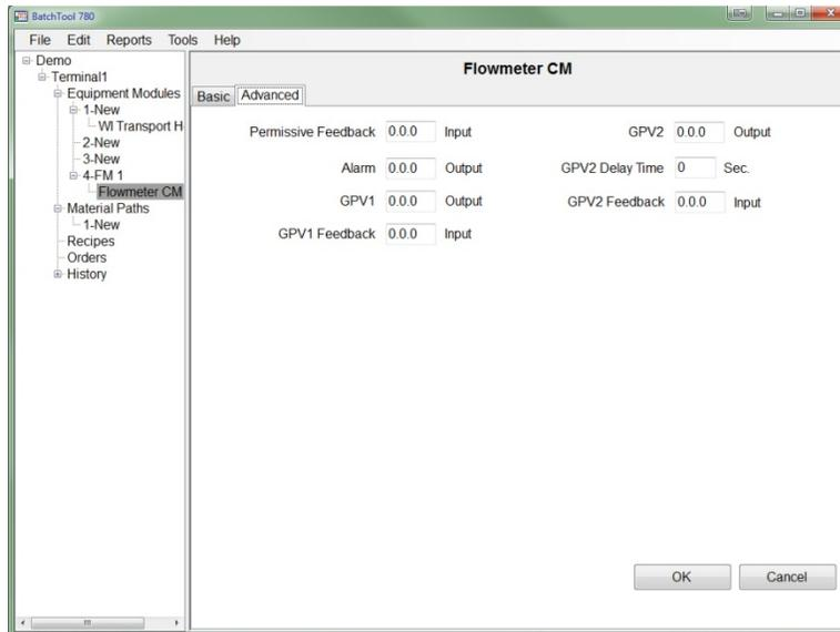
**Figure 9-20: Flow Meter Control Module, Advanced Tab**
