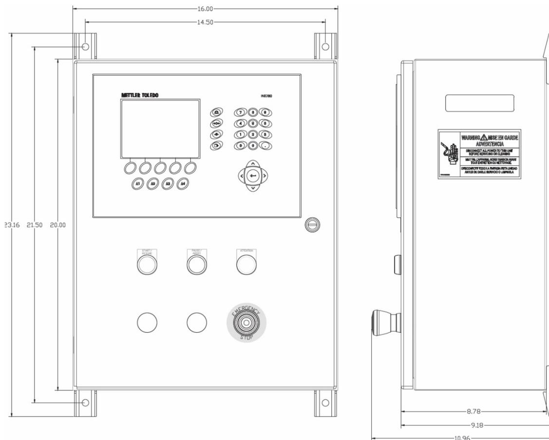
**Figure 1-9: Packaged IND780batch Dimensions, Front and Side**
