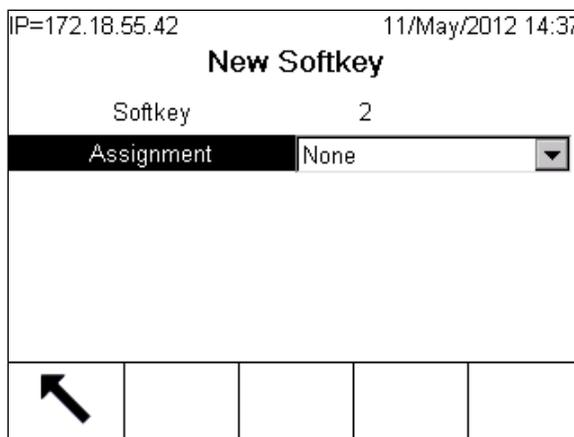
**Figure 3-21: New Softkey Configuration Screen**
