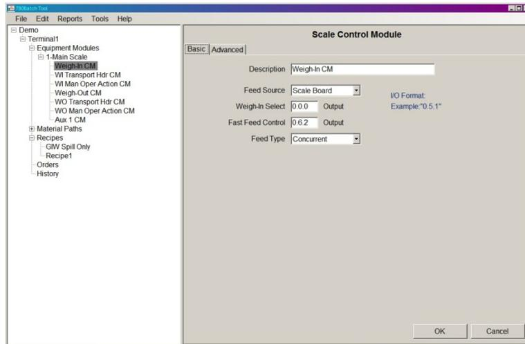
Figure 9-3: Weigh-In CM, Basic Tab
