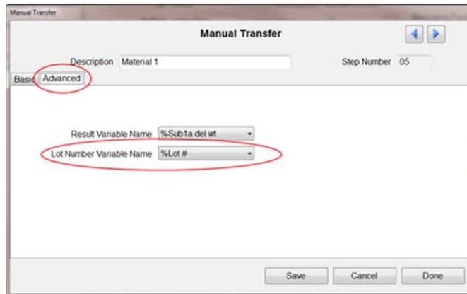
**Figure 14-14: Associating the Batch Variable with a Material**
