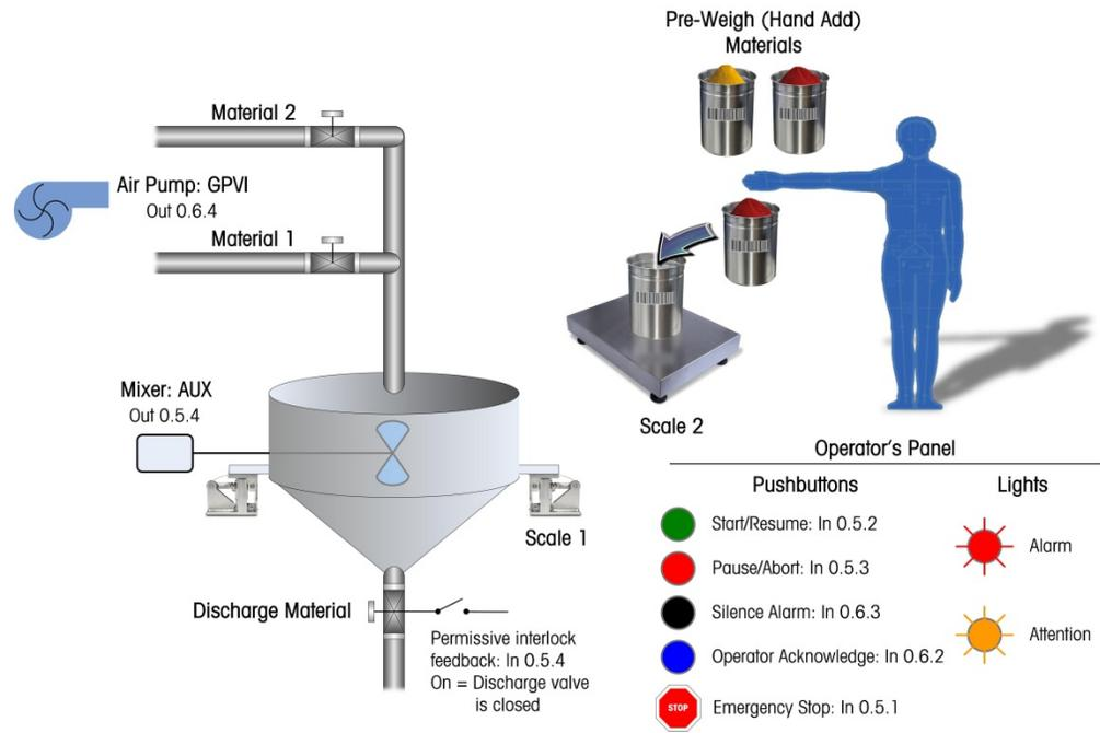
Figure 15-7: IND780batch Two-Scale System Diagram
