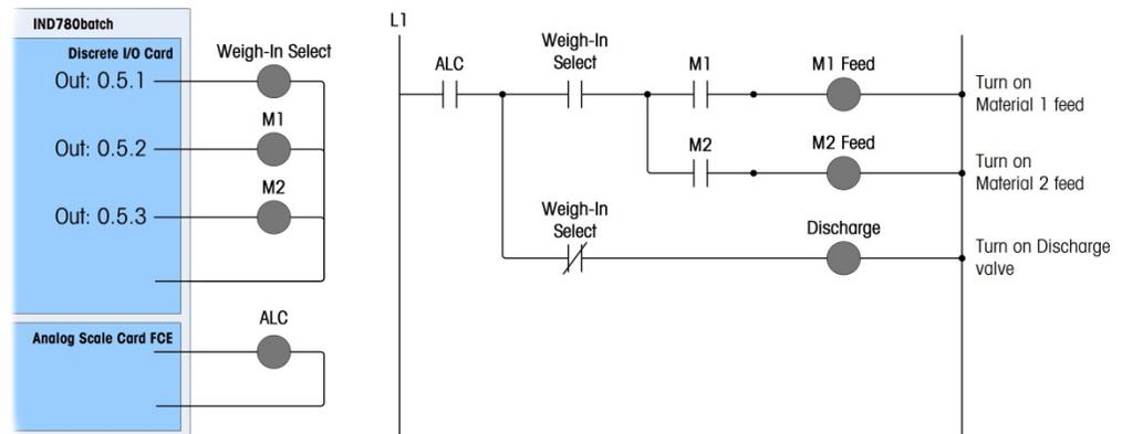
Figure 15-8: IND780batch Two-Scale System – Control Logic Diagram
