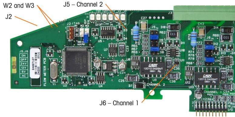
**Figure E-4: Flow Meter Interface Board Jumper Locations**
