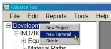
**Figure 8-2: Opening a New Terminal**
