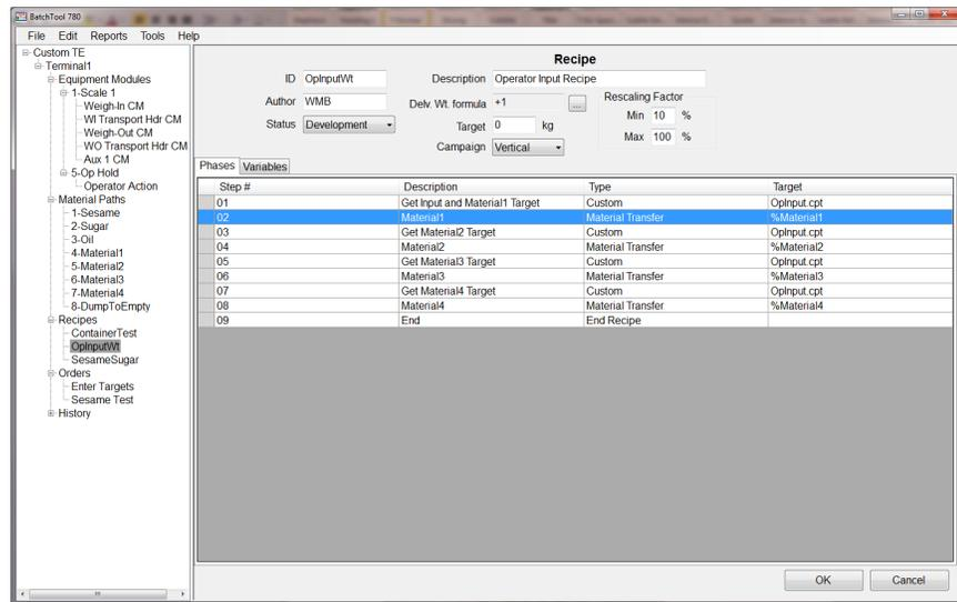
Figure 15-25: Weight Input Recipe, Phases Tab
