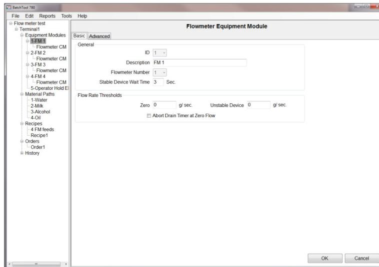
Figure 9-17: Flow Meter Equipment Module, Basic Tab
