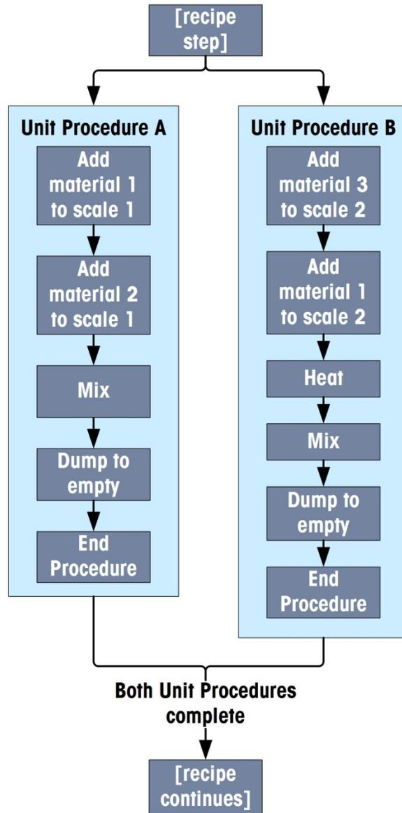
Figure 2-5: Example of Unit Procedure
