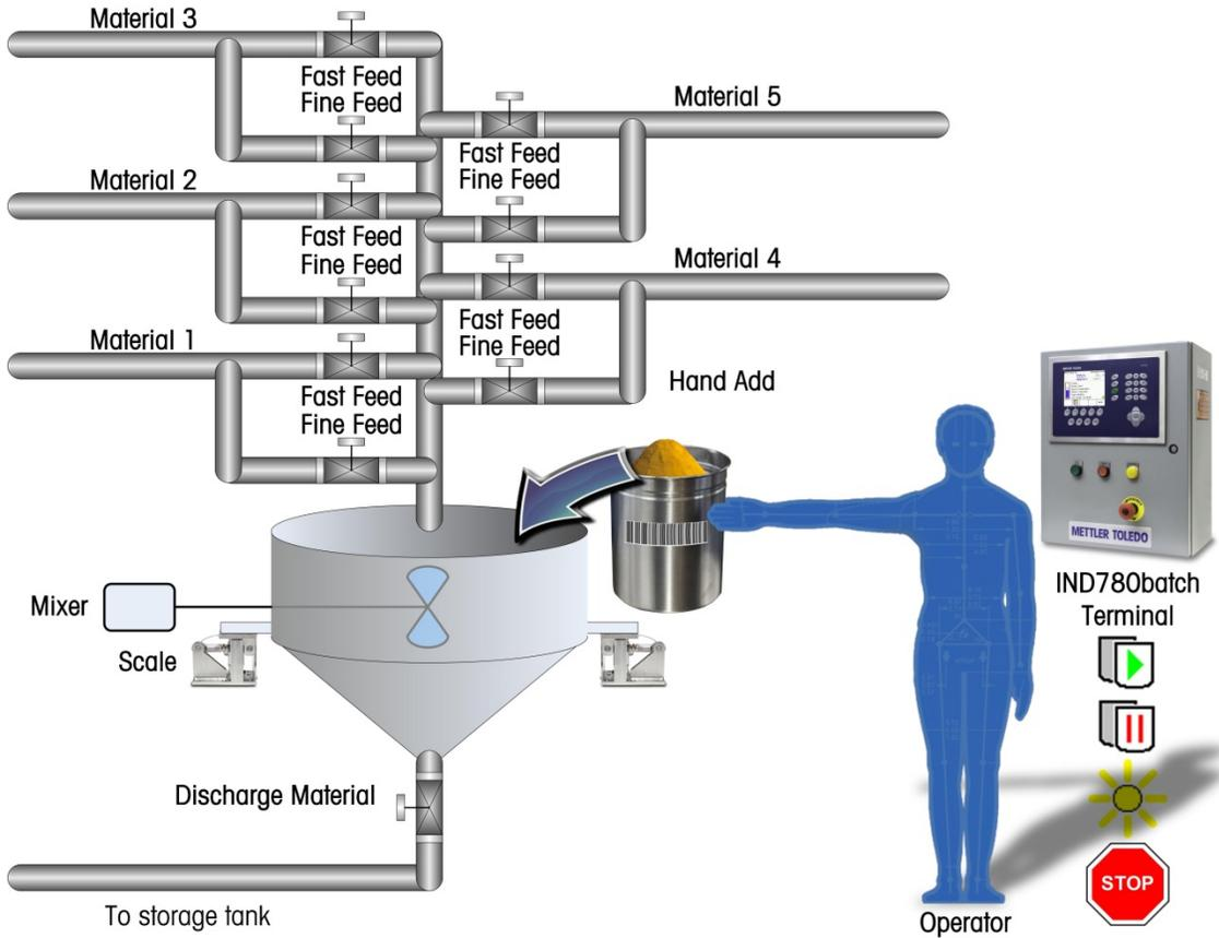
Figure 1-10: Automatic Batching System, Six Materials
