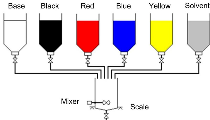
**Figure 12-9: Hopper System for Paint Batching**
