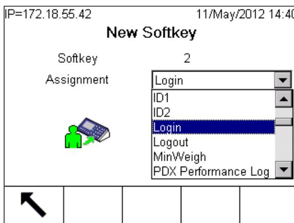
**Figure 3-22: Softkey Assignment Drop-Down List**
