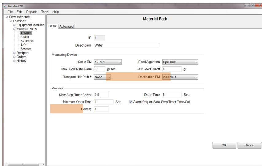
Figure 10-3: Flow Meter Material Path, Basic Tab
