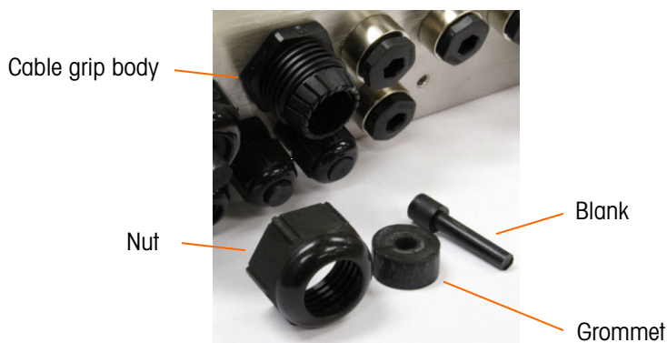
Figure A-22: Cable Gland Components
