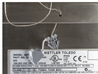
Figure A-99: Sealing Wire Threaded Through Cover and Clip
