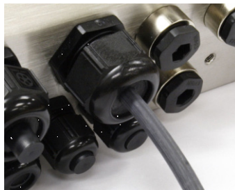
Figure A-26: Cable Grip Assembled
