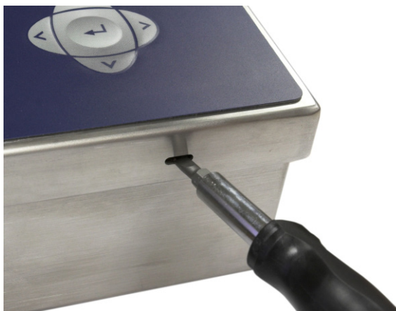
Figure A-2: Opening the Harsh Enclosure
