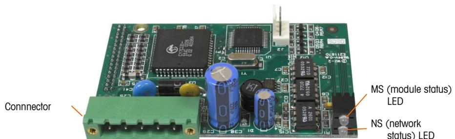
**Figure 4-2: DeviceNet Option Board Components**
