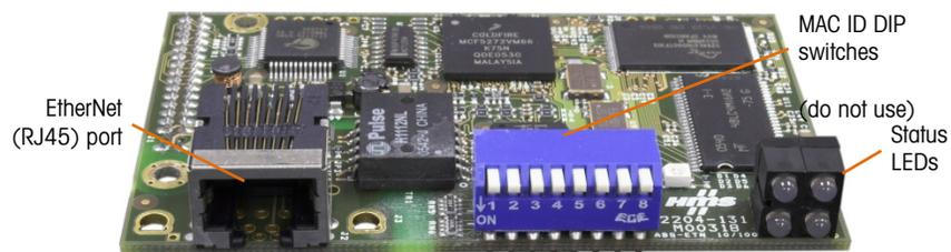
Figure 6-2: Ethernet / IP - Modbus TCP Option Board Components
