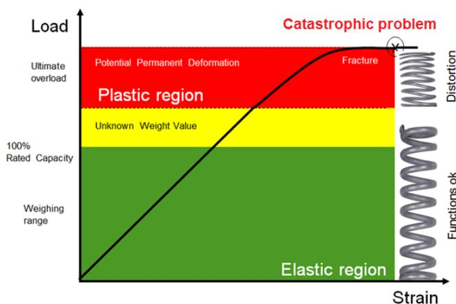
Figure 2-8: Load Cell Capacity Zones
