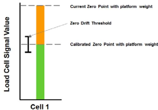
Figure 2-6: Zero Drift Monitoring
