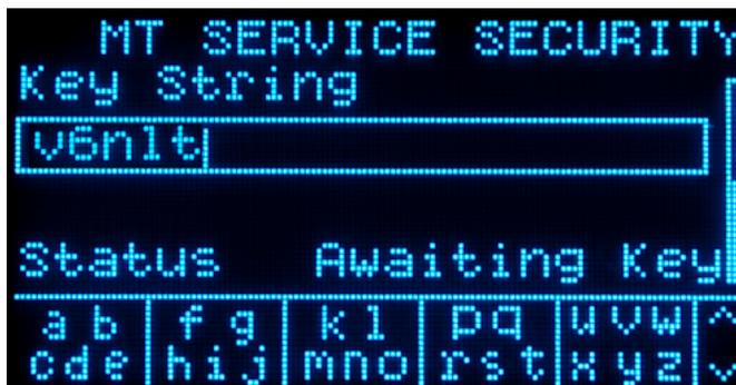
**Figure 3-10: Entry of InSite Key String into IND560 PDX**
