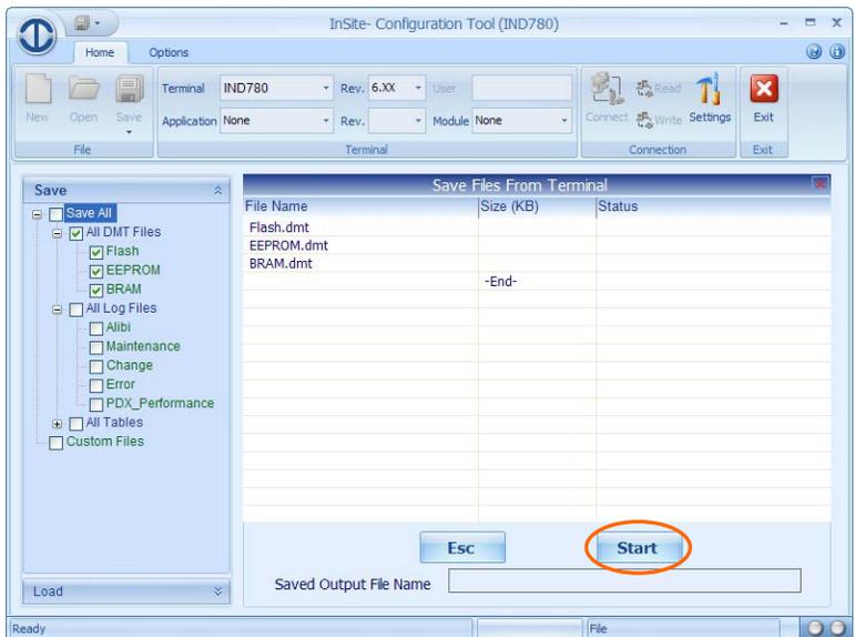
Figure 3-6: Starting the Save Process
