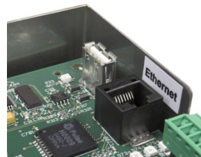
Figure 2-3: IND780 Ethernet Port
