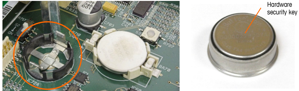
Figure 1-2: IND780 Hardware Key Socket on Mother Board
