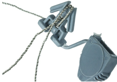
Figure A-96: Wire Looped Around Seal
