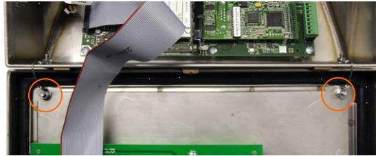
Figure A-7: Ground Strap Attachment Locations
