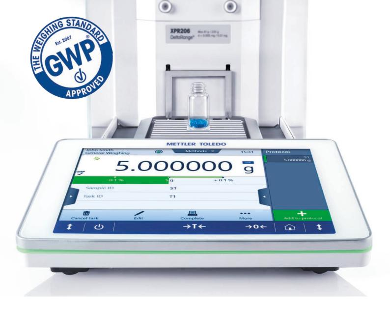
Your METTER TOLEDO service technician uses the information from your GWP® Verification and the balance calibration to program the built-in GWP Approved quality assurance function. GWP Approved prompts you to carry out calibration and routine balance tests in accordance with your specific accuracy requirements. A record of all tests is maintained that is suitable for audit purposes. Your benefit: GWP Approved documents the proven validity of every single result over the balance lifetime.
