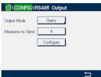
The Query option allows the RS485 output to be configured for output to either a PC or PLC only when the data is requested. The output data configured at the M800 will be sent when the command „D00Z” is received by the M800 over the RS485 communication line.
