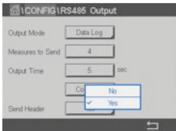
**Output Time** defines the time between each output cycle. The output time may be configured for from 1 to 3600 seconds, or from 1 to 60 minutes (1 hour).
