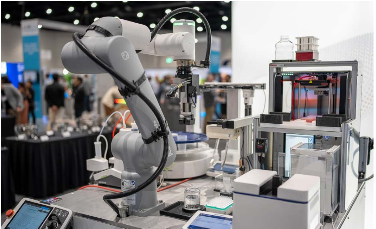
Figure 2: A cobot working with multiple instruments in a single workflow.
