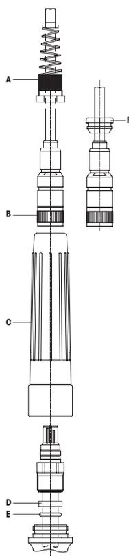
Removal of electrode/sensor from InFit 761e housing.
