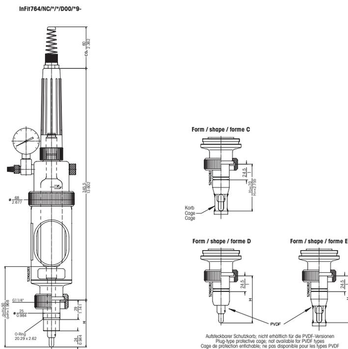
Different shapes for the lower part of the immersion tube.
