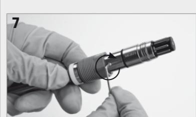
**E Instructions for the interior body exchange of the CO<sub>2</sub> sensors InPro® 5000**
