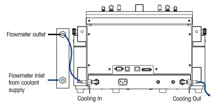
The instrument is delivered with two PVC industrial tubes. If you use the flowmeter, you need a third piece which can be cut away from one of the delivered tubes.
