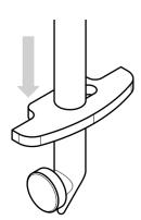
2 Turn the stirrer blade so that its cut-out aligns with the glass spike and move it over the glass spike.
