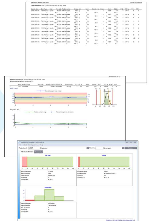
Devices in the FreeWeigh.Net® quality control system are connected to the in-house computer network. All the data recorded here is stored in the central data server. The immediately updated statistics are transmitted as a confirmation to the test sites and automatically displayed on the monitoring systems.
