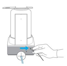
6. Load Rainin UNV 250  $\mu\text{L}$  tips or a glass (Pasteur) pipette onto appropriate adapter
