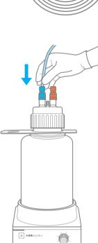
7. Firmly push the filter-end of the blue airflow tube onto the port labelled "Inlet" on the rear of the base unit. The filter picture points to the correct port.
