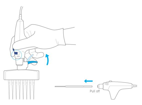
Figure 3: Ejecting Tips or removing the Pasteur pipette
